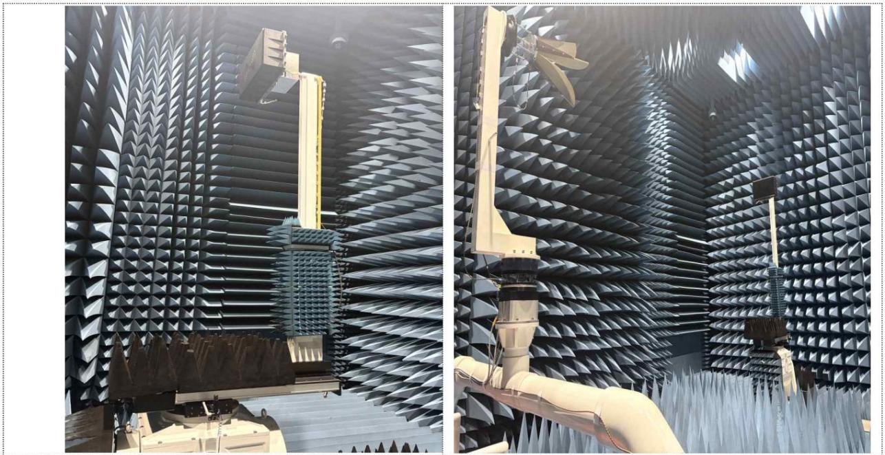
[Figure 2, 3] Antenna performance verification environment
