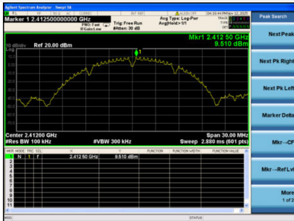
802.11b LOW CHANNEL, CARRIER LEVEL
