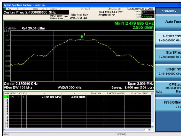
GFSK (BLE 1Mbps) HIGH CHANNEL, CARRIER LEVEL
