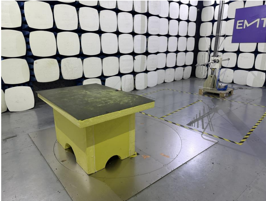
Spurious Emission Test Setup (Below 1GHz)
