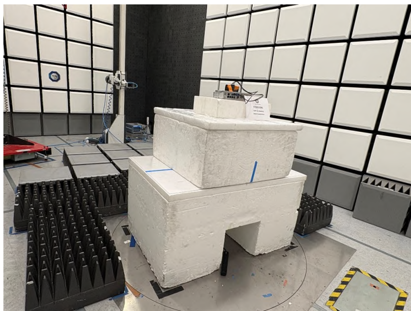
Radiated Emissions 8GHz to 18GHz Back View
