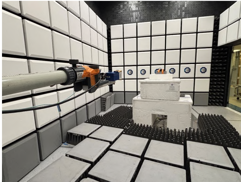
Radiated Emissions 26GHz to 40GHz Front View
