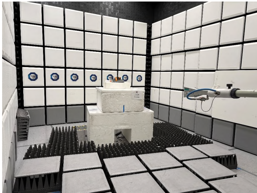
Radiated Emissions 8GHz to 18GHz Front View
