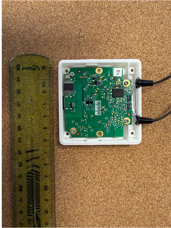
Front view of main PCBA in the command panel casing
