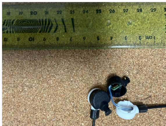
View of buffer PCBA in the earbud casing
