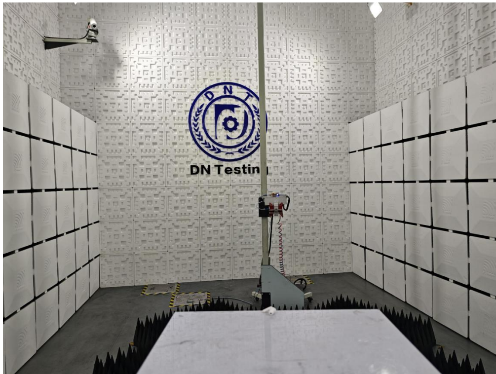
Radiated Emission Test View|(Above 1G)
