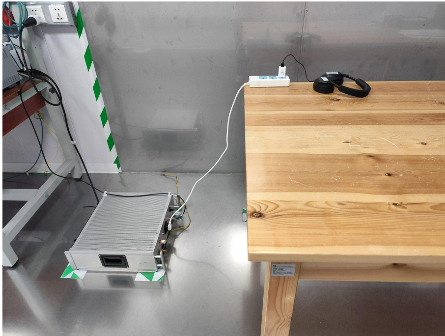
Conducted Emission at AC power line
