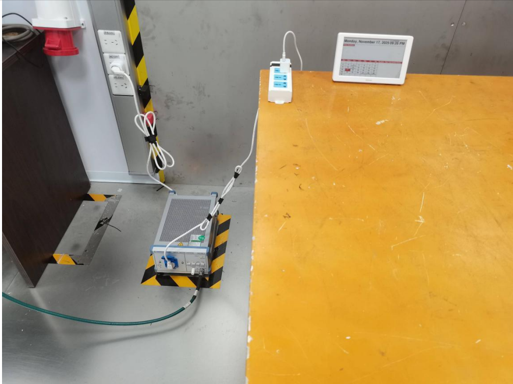
Radiated Spurious Emission, 9KHz~30MHz
