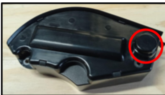
IoT box protecting cap circled in red
