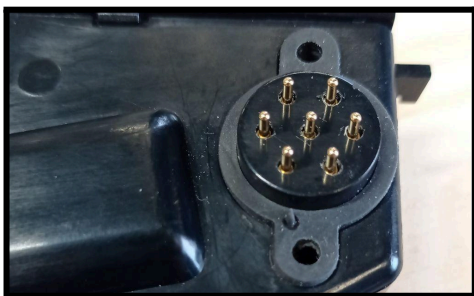
IoT box with connector gasket - OK
