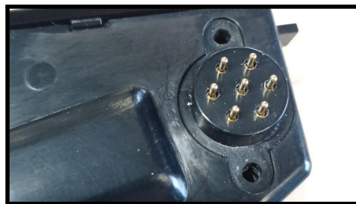
IoT box without connector gasket - NOK
