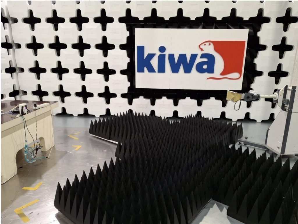
Photo 4 Photograph test setup conducted emissions, report section 3.2
