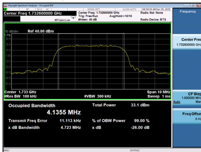
26dB&99% Occupied Bandwidth Plot on Channel 1513
