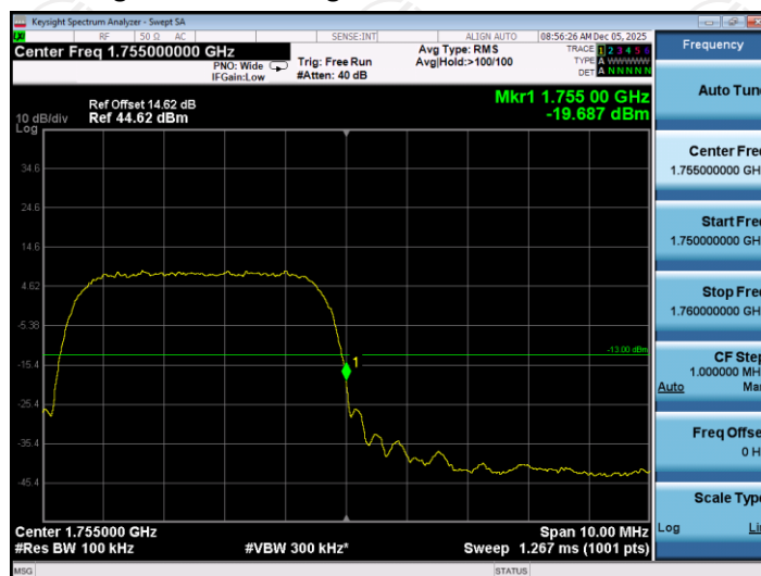
Higher Band Edge Plot on Channel 1513
