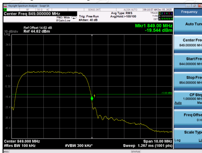
Higher Band Edge Plot on Channel 4233
