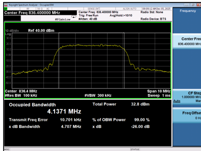
26dB&99% Occupied Bandwidth Plot on Channel 4233
