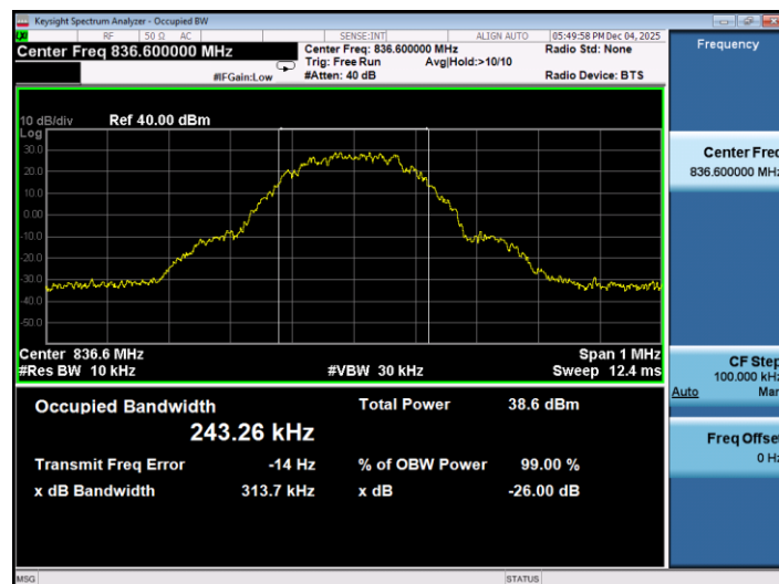
26dB&99% Occupied Bandwidth Plot on Channel 251
