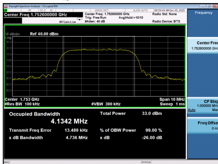
26dB&99% Occupied Bandwidth Plot on Channel 1513
