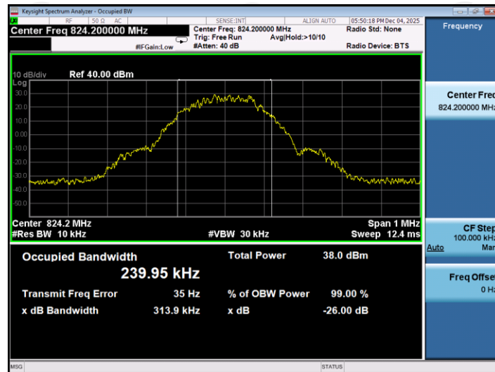
26dB&99% Occupied Bandwidth Plot on Channel 190
