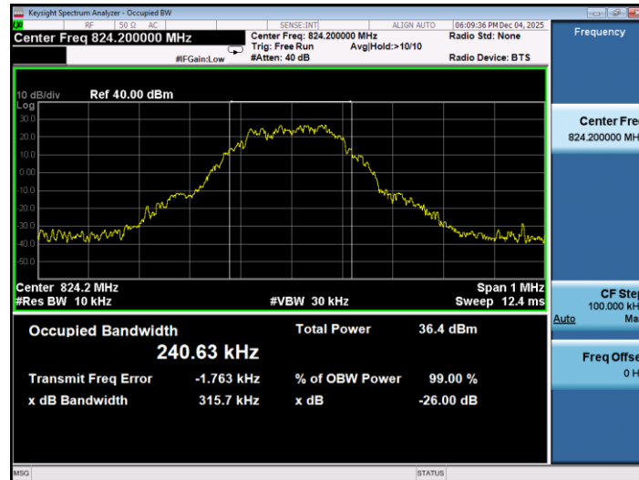
26dB&99% Occupied Bandwidth Plot on Channel 190
