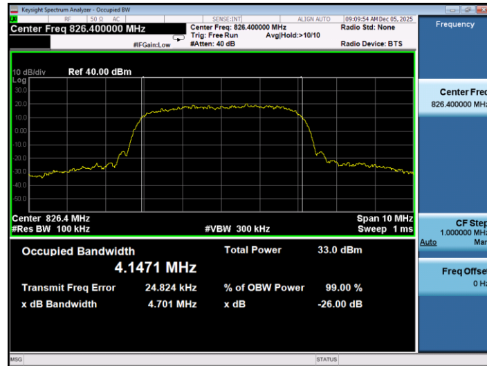
26dB&99% Occupied Bandwidth Plot on Channel 4182
