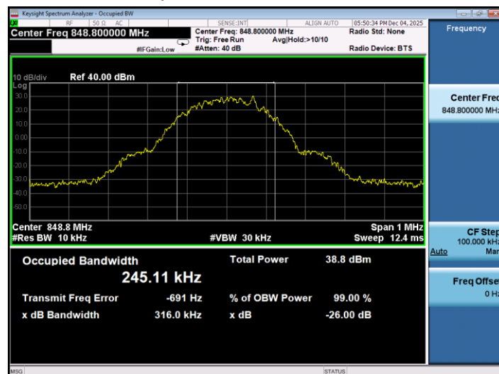
26dB&99% Occupied Bandwidth Plot on Channel 251
