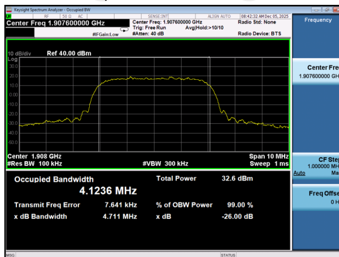
26dB&99% Occupied Bandwidth Plot on Channel 9538
