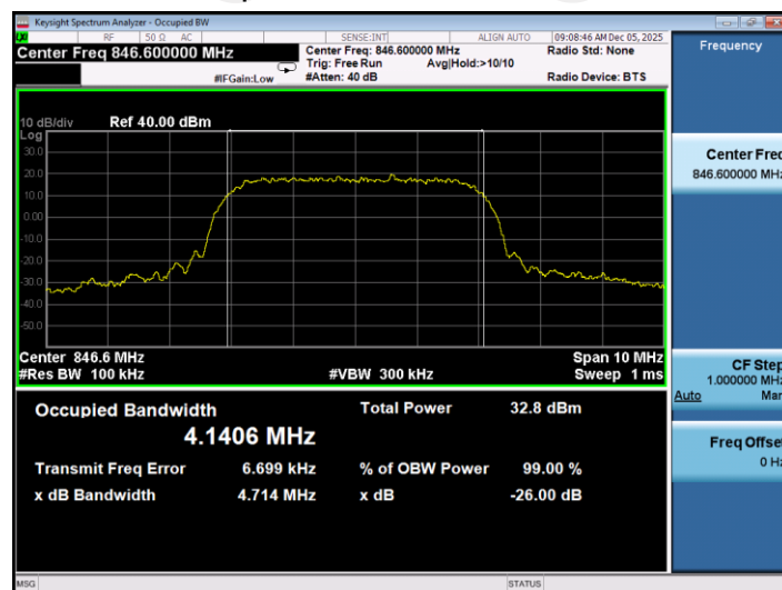
26dB&99% Occupied Bandwidth Plot on Channel 4233
