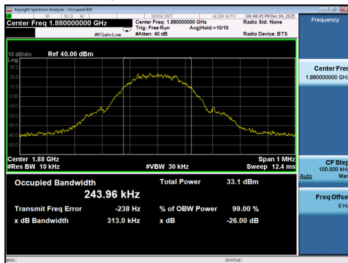
26dB&99% Occupied Bandwidth Plot on Channel 810
