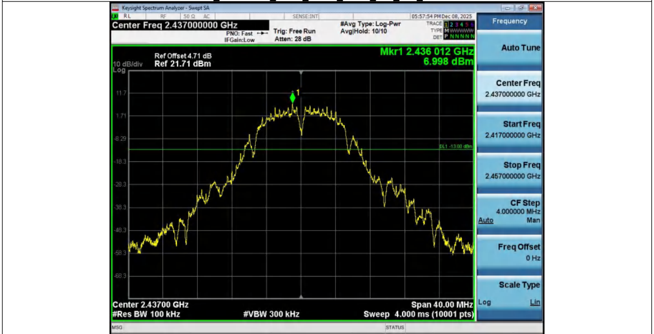
2 Spurious Emission NVNT_ANT1_802_11b_2437
