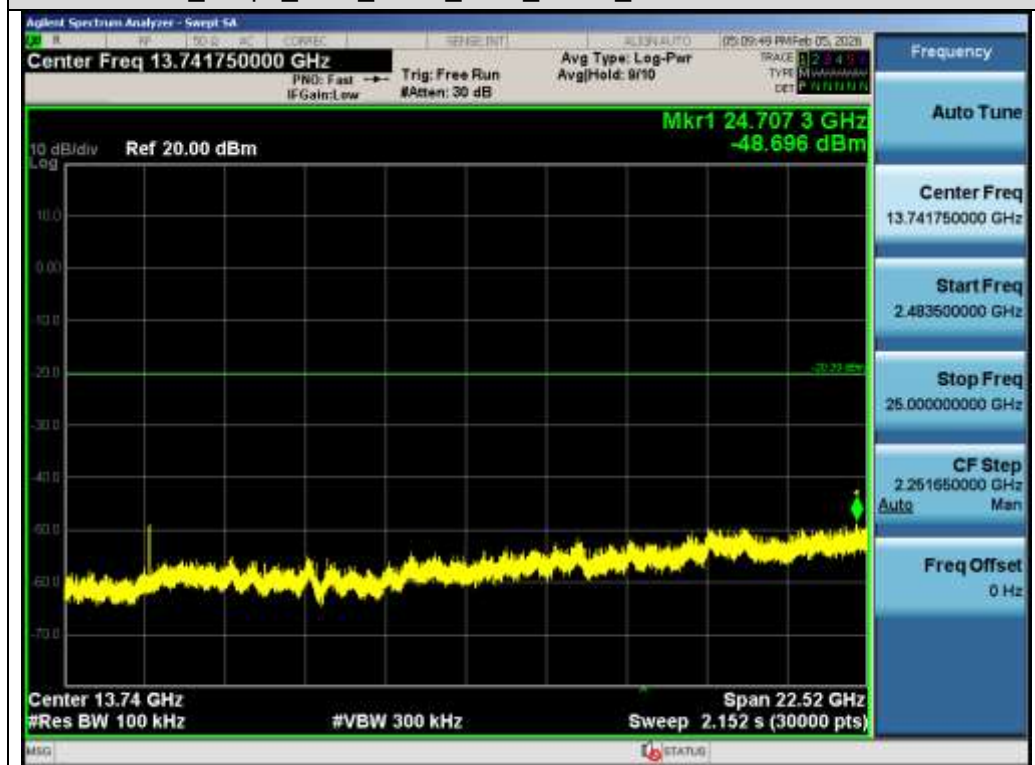
Test_Graph_2.4G_ANT1_2430_GFSK_Higher Band Emissions
