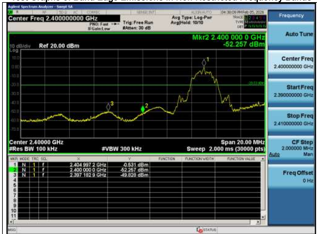
Test_Graph_2.4G_ANT1_2405_GFSK_Lower Band Edge Emissions
