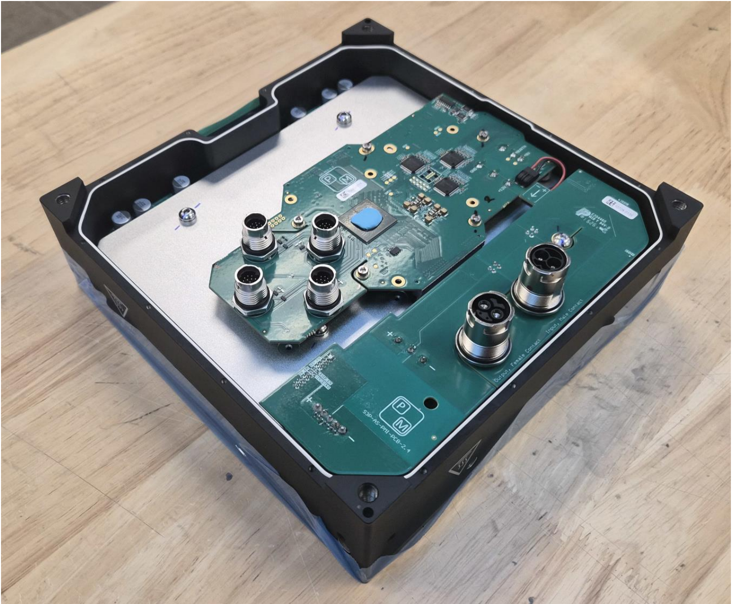
Isometric view of controller board installed in housing
