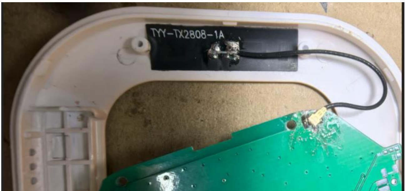
Figure 3 Assembly drawing (WIFI antenna)
