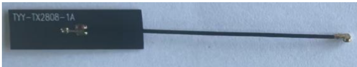
Figure 2 TYY-TX2808-1A WIFI Antenna finished product (wire length 55mm with 3rd generation terminals)
