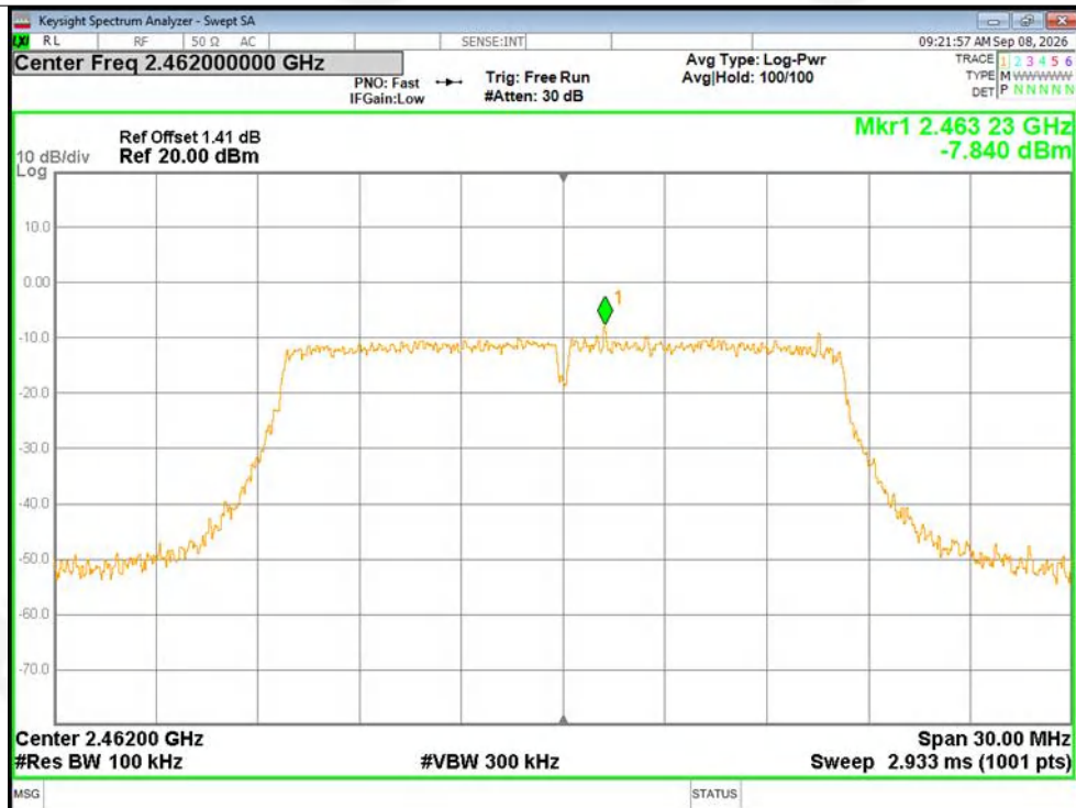
Tx. Spurious NVNT g 2462MHz Ant1 Ref
