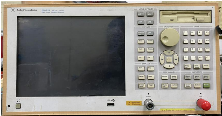
Agilent 5071B (S Parameter (RL/VSWR) Test Equipment
