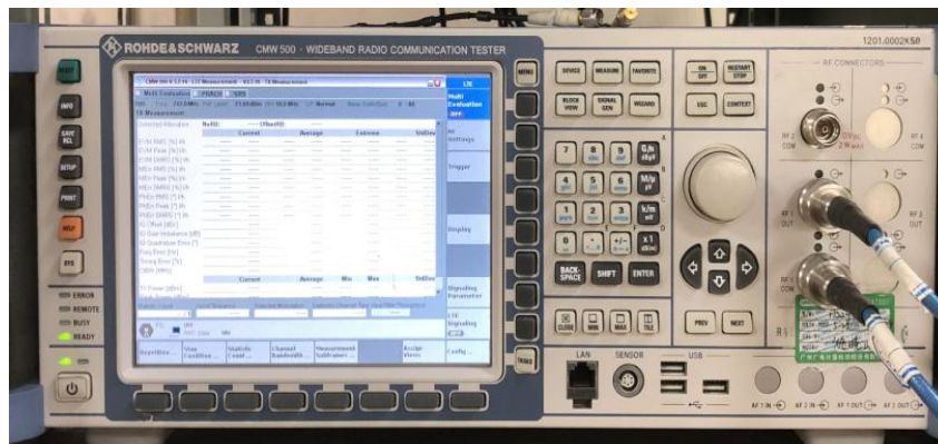
CMW 500 (2G/3G/4G Test Equipment)
