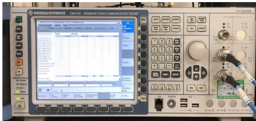
CMW 500 (2G/3G/4G Test Equipment)
