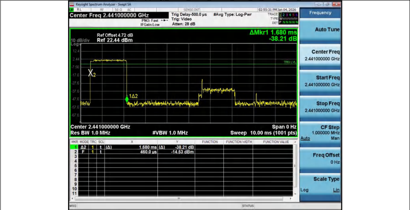
Dwell_Time (Hopping) NVNT_ANT1_3-DH3_2441_00_Accumulated
