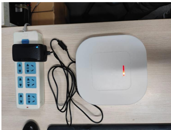
△ 10075423 Hub Power Connection
