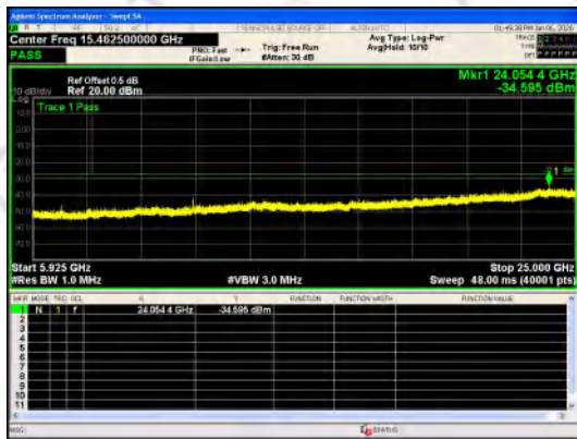
Spurious Emission:5925~25000.0 MHz IEEE 802.11n_Channel 157_20MHz_Antenna 0
