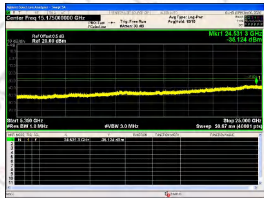
Spurious Emission:5350~25000.0 MHz IEEE 802.11n_Channel 48_20MHz_Antenna 0
