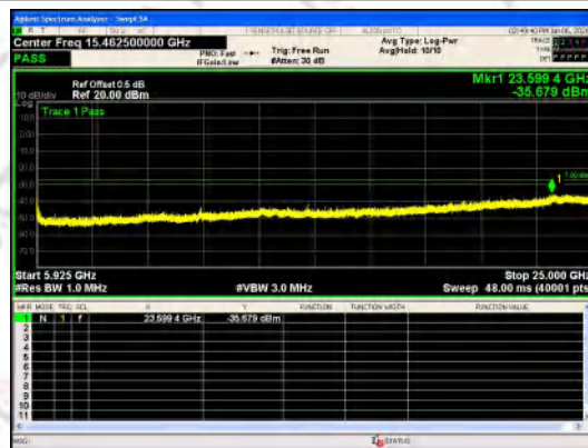
Spurious Emission:5925~25000.0 MHz IEEE 802.11ac_Channel 155_80MHz_Antenna
