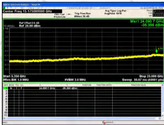
Spurious Emission:5350~25000.0 MHz IEEE 802.11a_Channel 36_20MHz_Antenna 0
