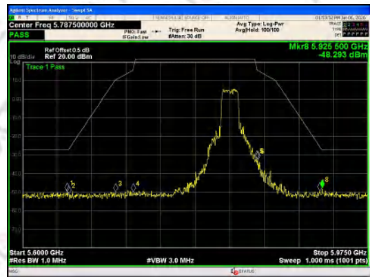
Out Of Band Emission IEEE 802.11n_Channel 165_20MHz_Antenna 0
