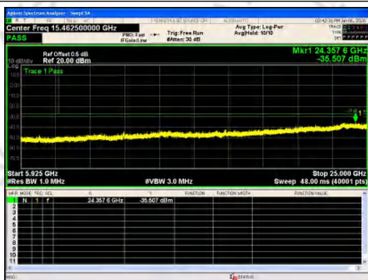
Spurious Emission:5925~25000.0 MHz IEEE 802.11ac_Channel 159_40MHz_Antenna 0
