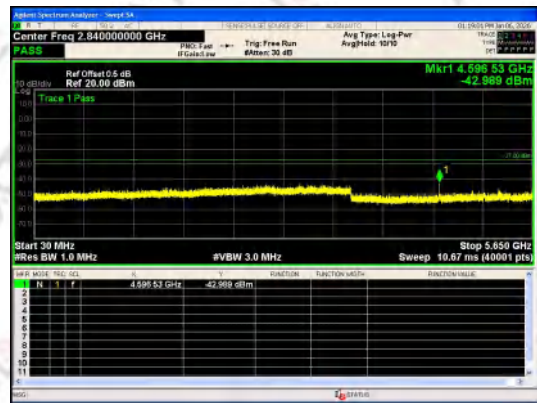
Spurious Emission:30.0~5650 MHz IEEE 802.11a_Channel 149_20MHz_Antenna 0
