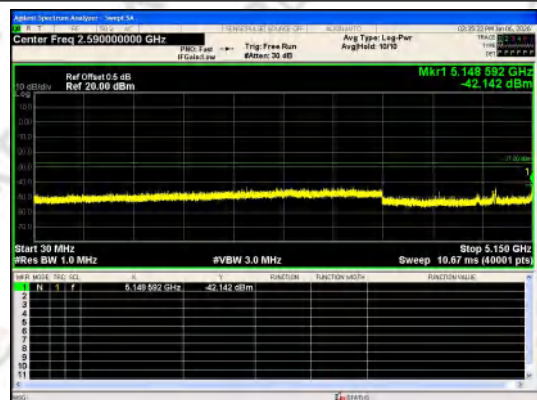
Spurious Emission:5350~25000.0 MHz IEEE 802.11ac_Channel 38_40MHz_Antenna 0
