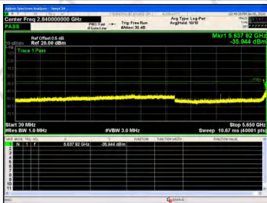
Spurious Emission:30.0~5650 MHz IEEE 802.11ac_Channel 155_80MHz_Antenna
