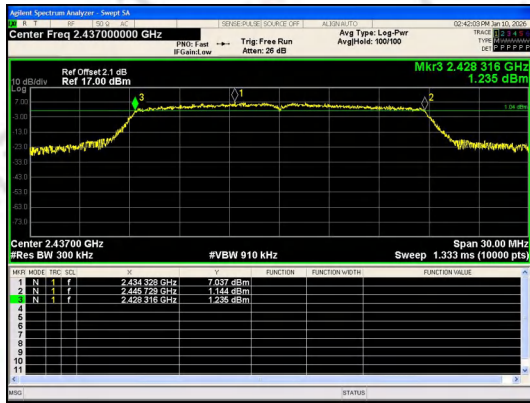
IEEE 802.11g_Channel 6_20MHz_Antenna 0
