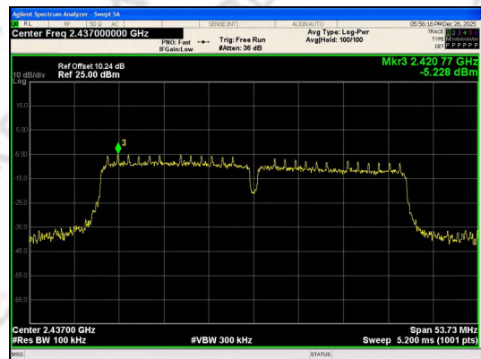
Out Of Band Emission IEEE 802.11n_Channel 3_40MHz_Antenna 0
