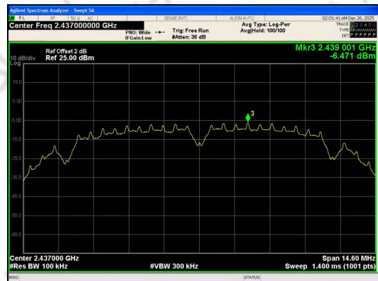
In-Band Reference Level IEEE 802.11b_Channel 6_20MHz_Antenna 0
