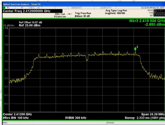
In-Band Reference Level IEEE 802.11g_Channel 1_20MHz_Antenna 0
