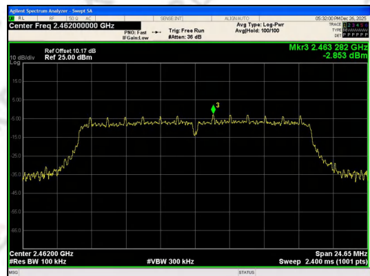
In-Band Reference Level IEEE 802.11g_Channel 6_20MHz_Antenna 0
