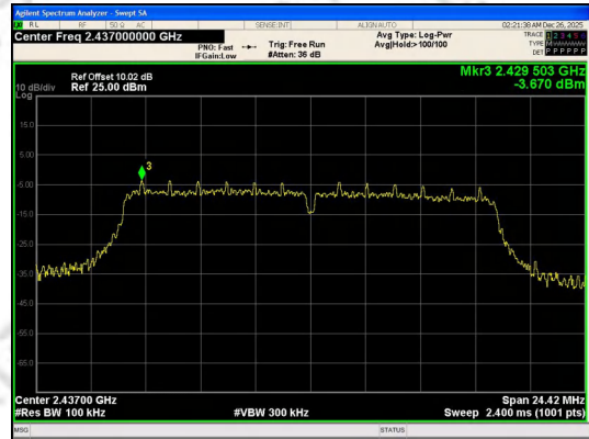
In-Band Reference Level IEEE 802.11g_Channel 6_20MHz_Antenna 0
