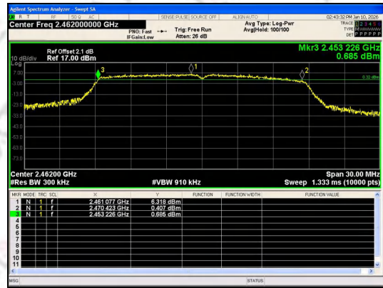
IEEE 802.11g_Channel 11_20MHz_Antenna 0
