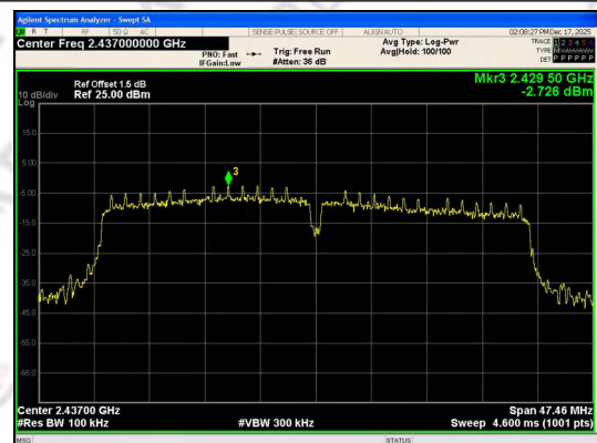
Out Of Band Emission IEEE 802.11n_Channel 3_40MHz_Antenna 0
