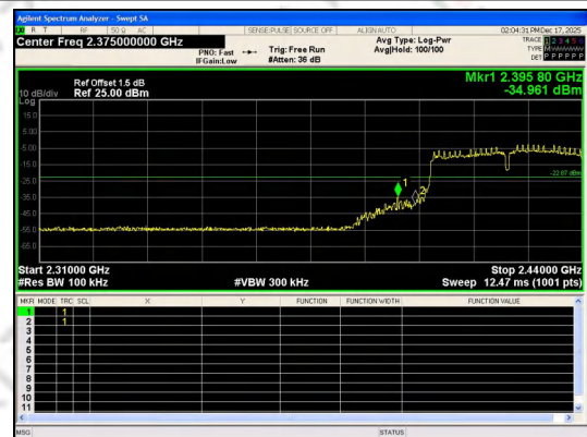
Out Of Band Emission IEEE 802.11n_Channel 3_40MHz_Antenna 0
