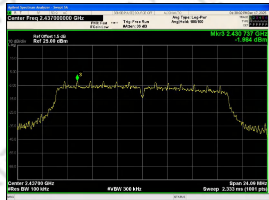
In-Band Reference Level IEEE 802.11g_Channel 6_20MHz_Antenna 0
