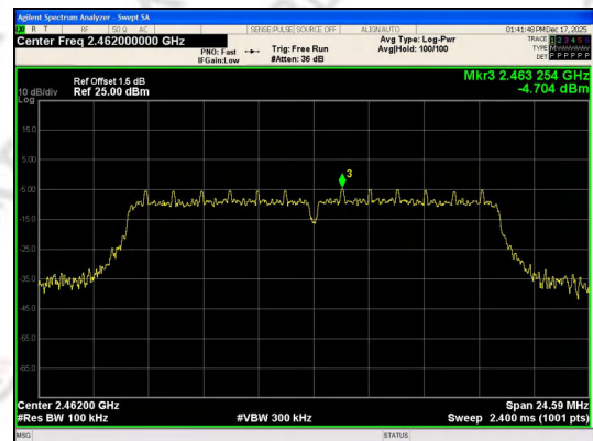
In-Band Reference Level IEEE 802.11g_Channel 6_20MHz_Antenna 0
