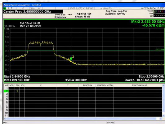
Out Of Band Emission IEEE 802.11n_Channel 11_20MHz_Antenna 0
