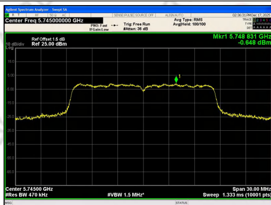
IEEE 802.11a_Channel 149_20MHz_Antenna 0
