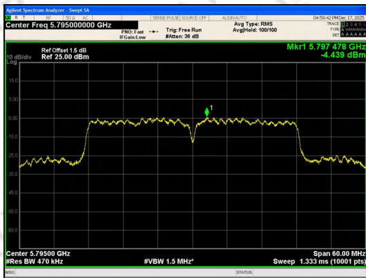
IEEE 802.11ac_Channel 159_40MHz_Antenna 0
