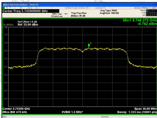
IEEE 802.11ac_Channel 149_20MHz_Antenna 0
