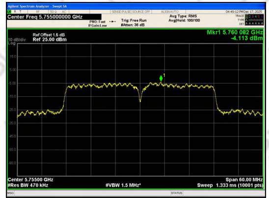
IEEE 802.11ac_Channel 151_40MHz_Antenna 0
