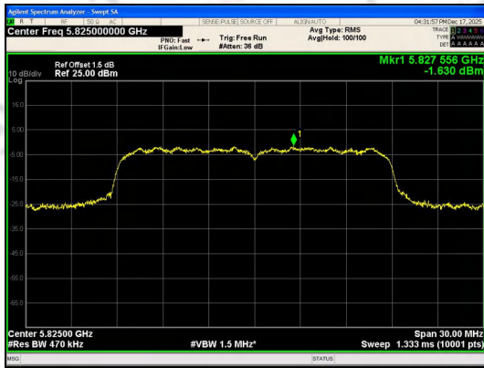
IEEE 802.11ac_Channel 165_20MHz_Antenna 0
