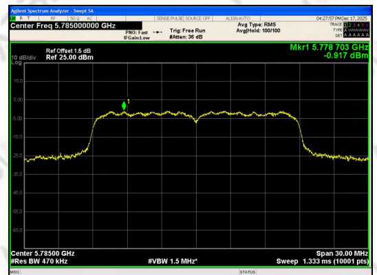
IEEE 802.11ac_Channel 157_20MHz_Antenna 0
