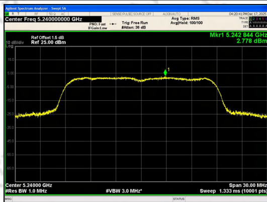
IEEE 802.11ac_Channel 48_20MHz_Antenna 0
