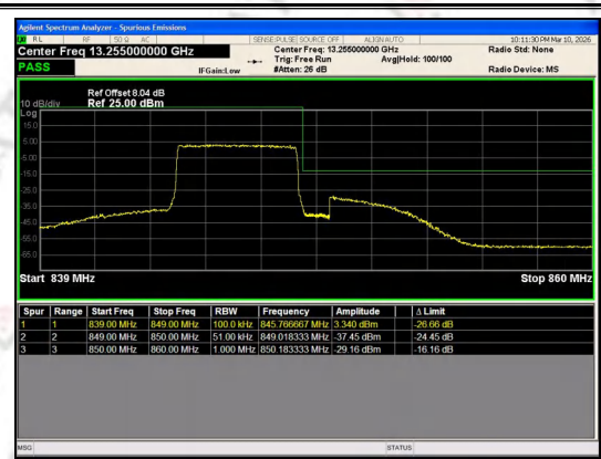
Band 5 5MHz/846.5/High 16QAM 25@0
