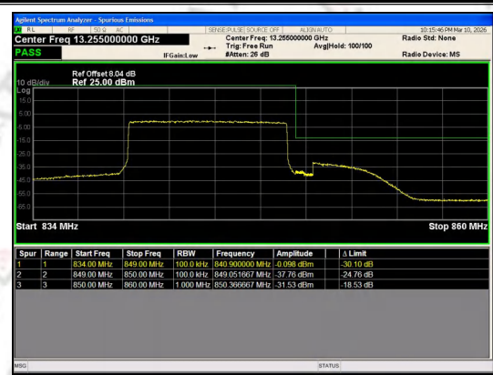
Band 5 10MHz/844.0/High 16QAM 50@0
