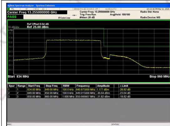
Band 5 10MHz/844.0/High QPSK 1@0
