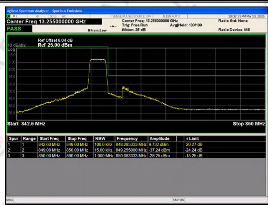
Band 5 1.4MHz/848.3/High 16QAM 6@0
