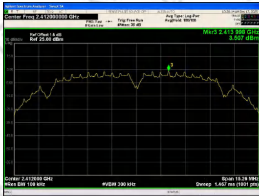
In-Band Reference Level IEEE 802.11b_Channel 1_20MHz_Antenna 0
