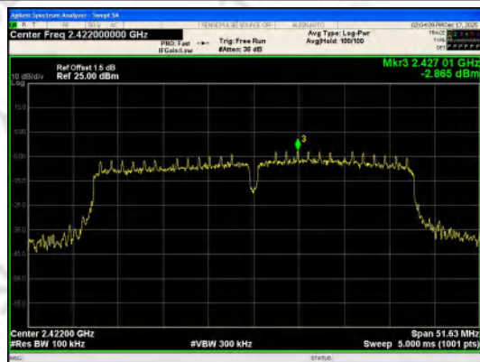
In-Band Reference Level IEEE 802.11n_Channel 3_40MHz_Antenna 0
