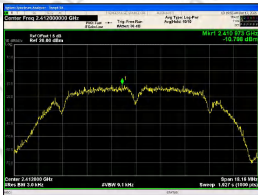
IEEE 802.11b_Channel 1_20MHz_Antenna 0
