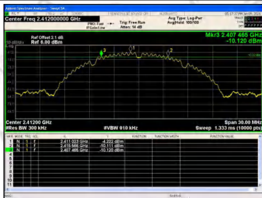
IEEE 802.11b_Channel 1_20MHz_Antenna 0
