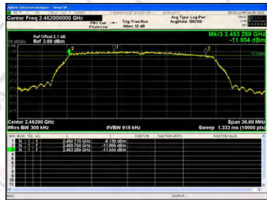
IEEE 802.11g_Channel 11_20MHz_Antenna 0
