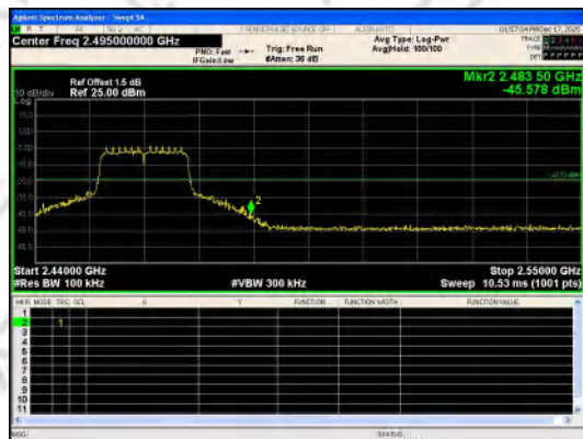
Out Of Band Emission IEEE 802.11n_Channel 11_20MHz_Antenna 0
