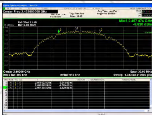
IEEE 802.11b_Channel 11_20MHz_Antenna 0
