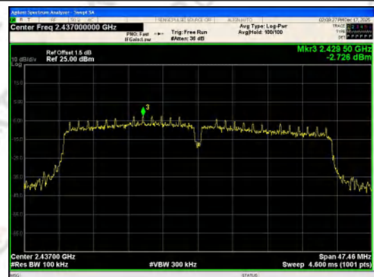
Out Of Band Emission IEEE 802.11n_Channel 3_40MHz_Antenna 0
