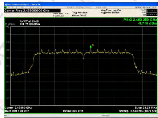
In-Band Reference Level IEEE 802.11n_Channel 11_20MHz_Antenna 0
