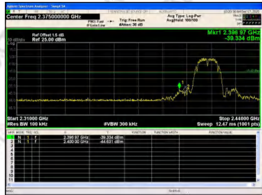
Out Of Band Emission IEEE 802.11b_Channel 1_20MHz_Antenna 0
