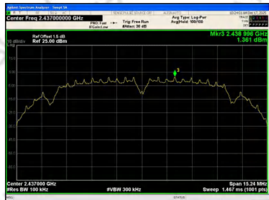
In-Band Reference Level IEEE 802.11b_Channel 6_20MHz_Antenna 0
