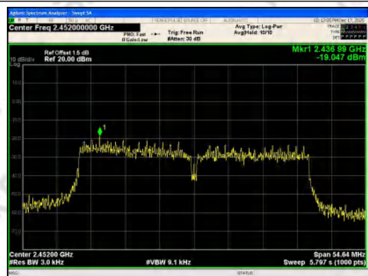
IEEE 802.11n_Channel 9_40MHz_Antenna 0
