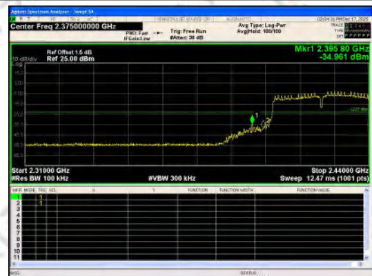
Out Of Band Emission IEEE 802.11n_Channel 3_40MHz_Antenna 0
