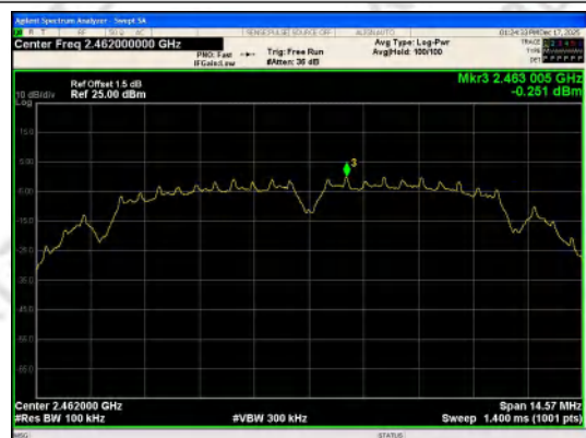
In-Band Reference Level IEEE 802.11b_Channel 11_20MHz_Antenna 0
