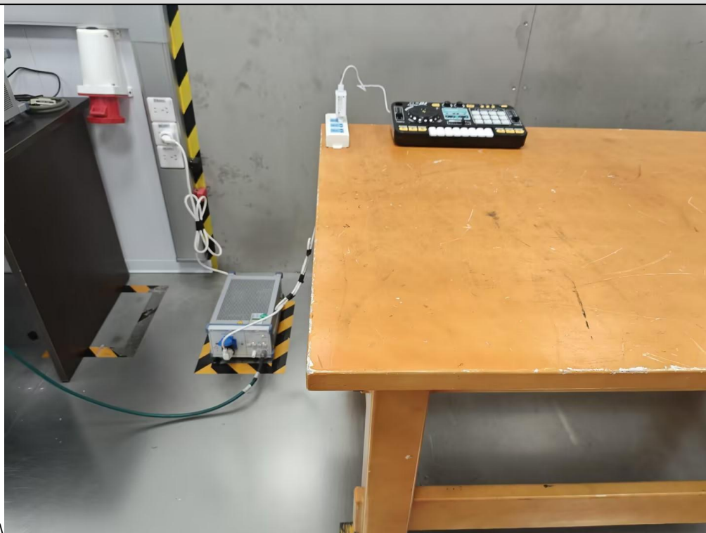
Radiated Spurious Emission Below 1GHz
