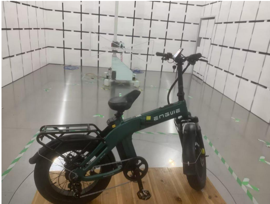
Field Strength of Radiated Emission-Below 1GHz
