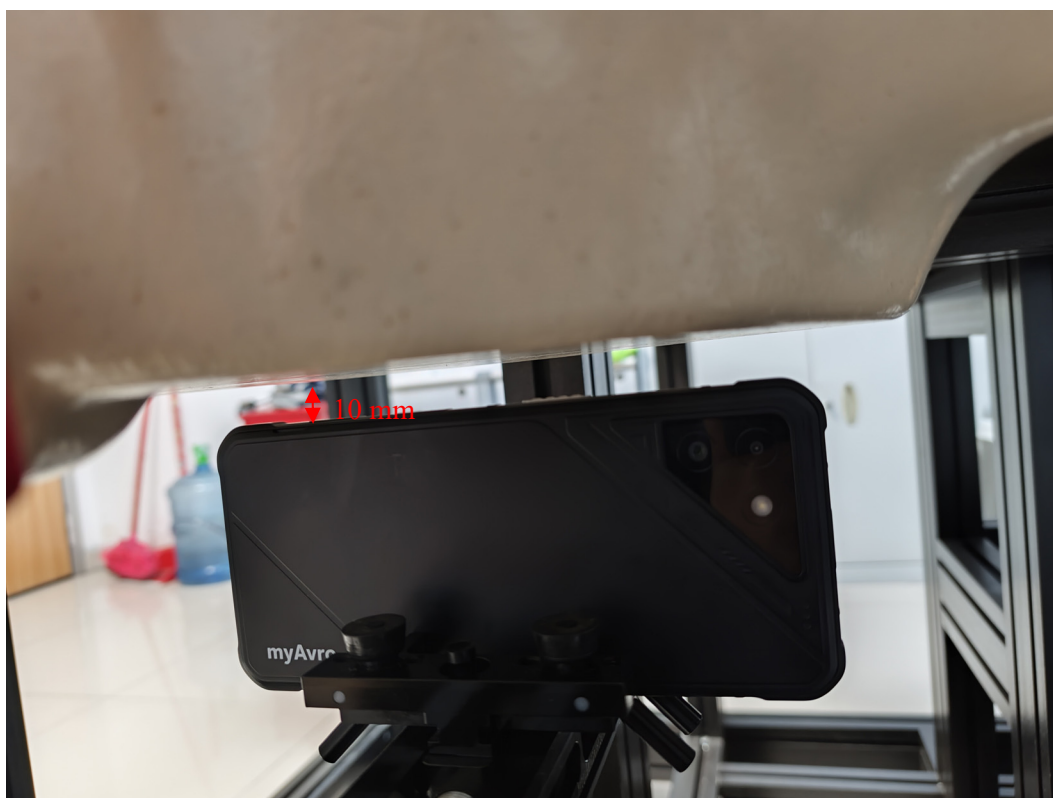
ANT5 Body Top Setup Photo (10 mm)
