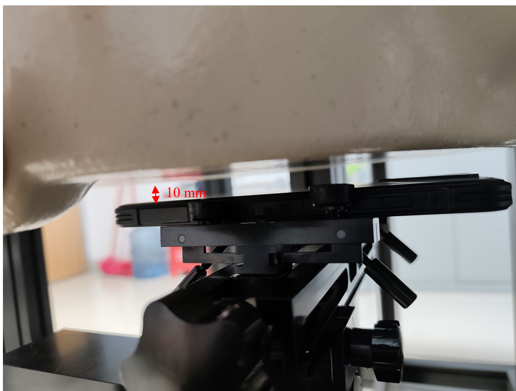
ANT1/2 Body Back Setup Photo (10 mm)
