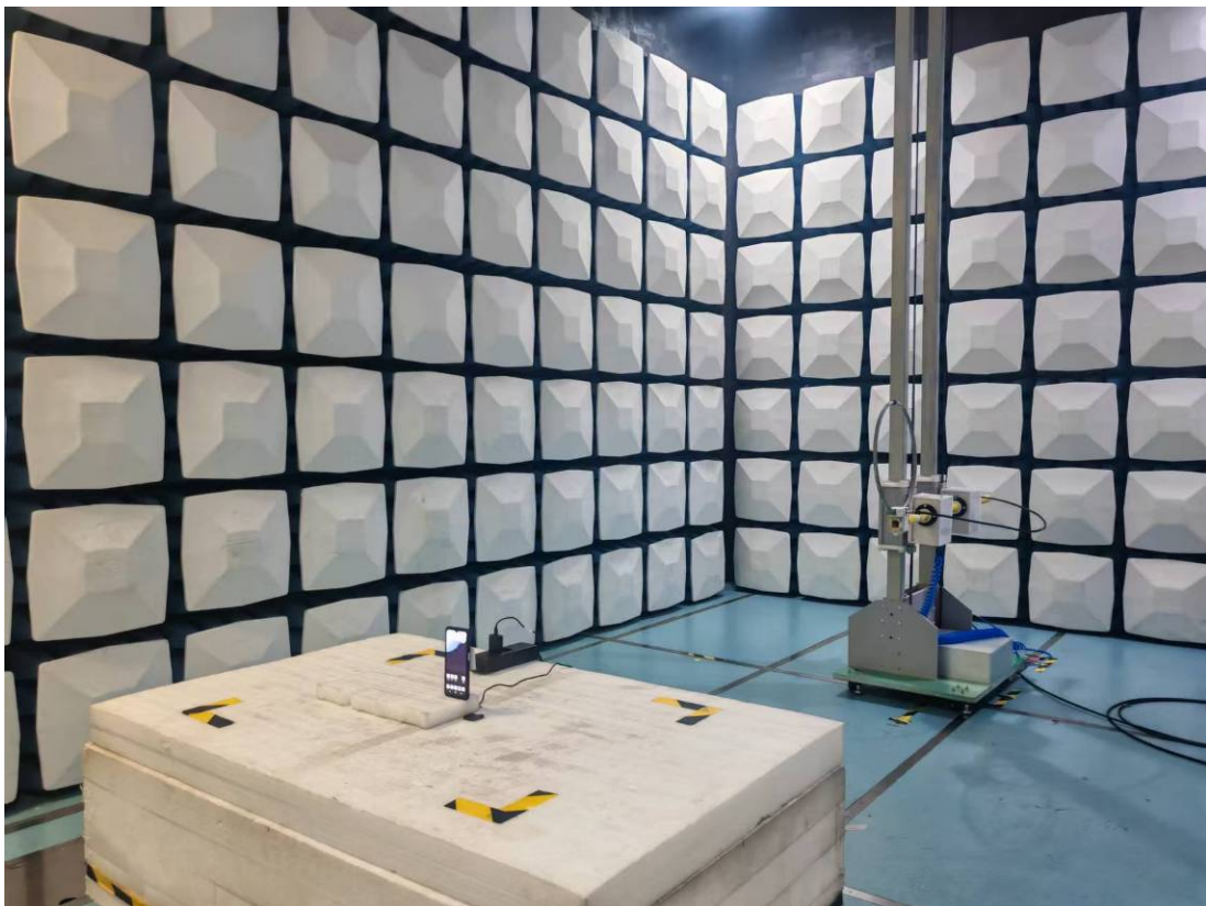
Radiated Emission 9k-30MHz Perpendicular View
