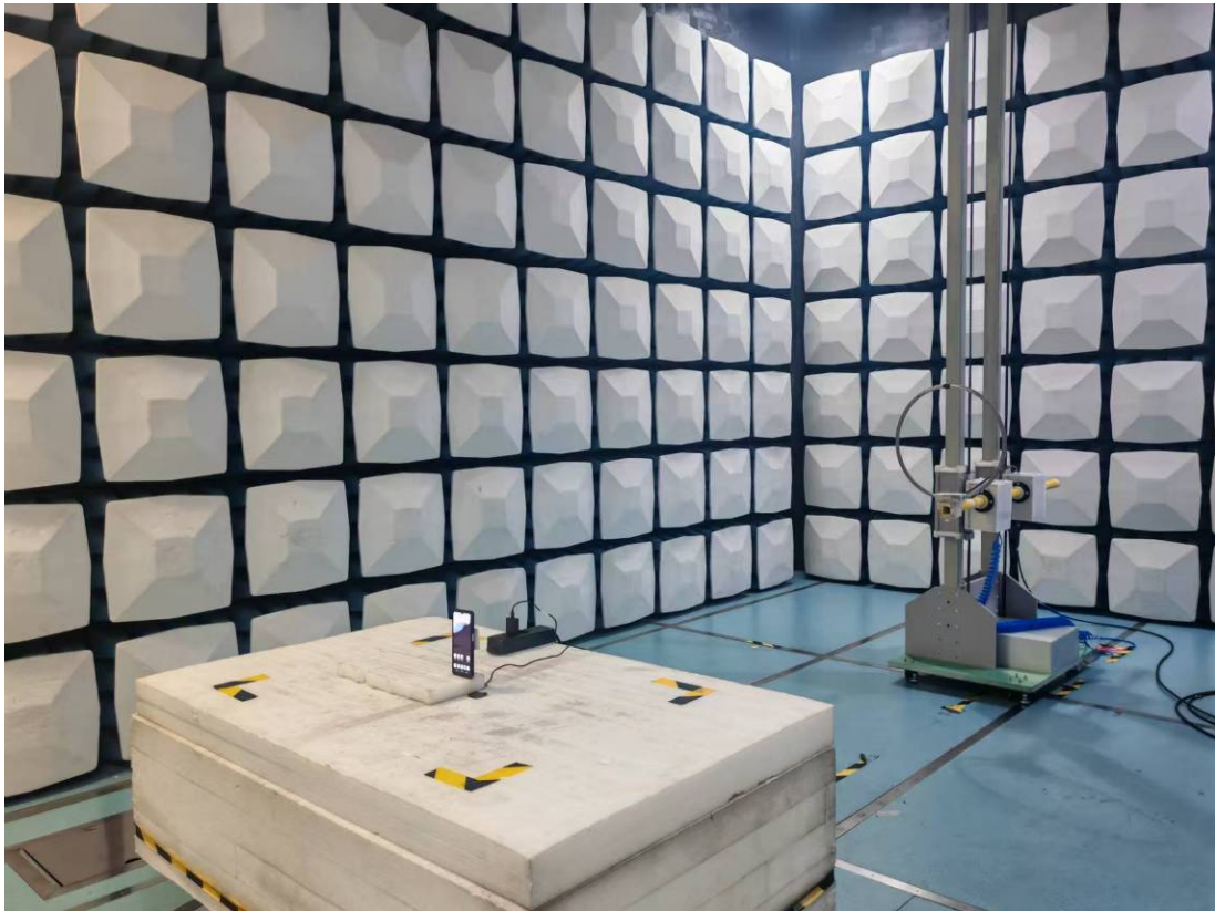
Radiated Emission 9k-30MHz Perpendicular View
