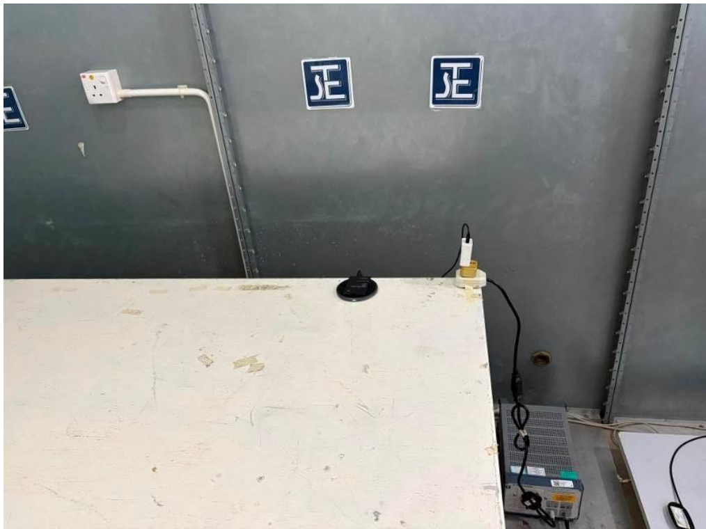
Measurement of Conducted Emission Test Set Up
