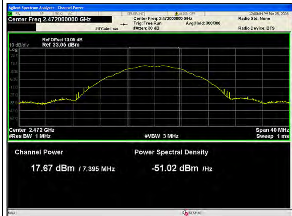
Peak Power NVNT b 2472MHz Ant2 SISO
