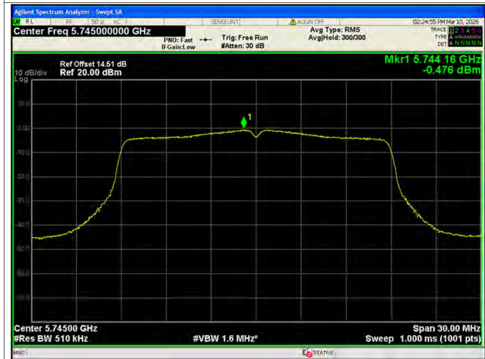
PSD NVNT n20 5745MHz Ant2 SISO
