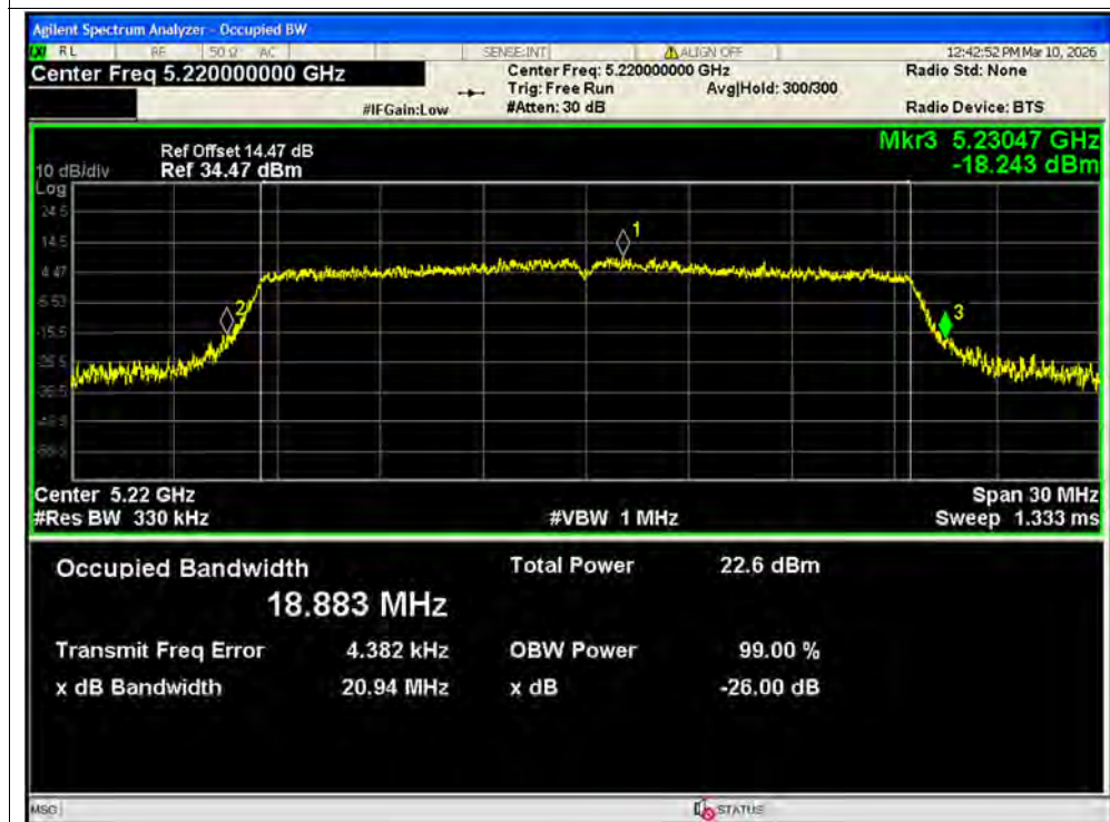
-26dB Bandwidth NVNT ax20 5220MHz Ant1 SISO
