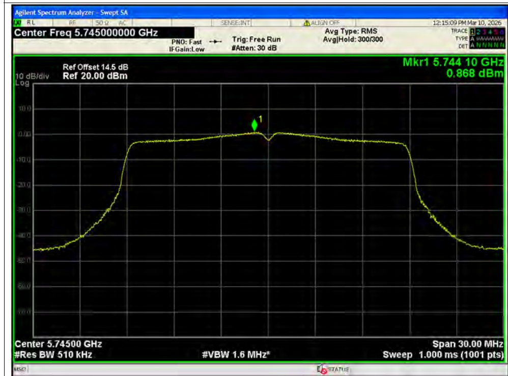
PSD NVNT n20 5745MHz Ant1 SISO
