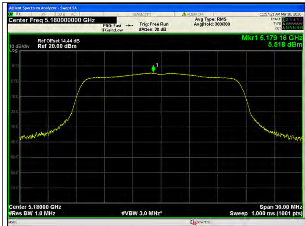
PSD NVNT a 5180MHz Ant1 SISO
