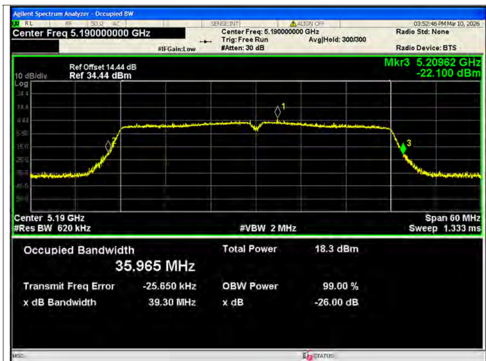
-26dB Bandwidth NVNT ac40 5190MHz Ant1 MIMO
