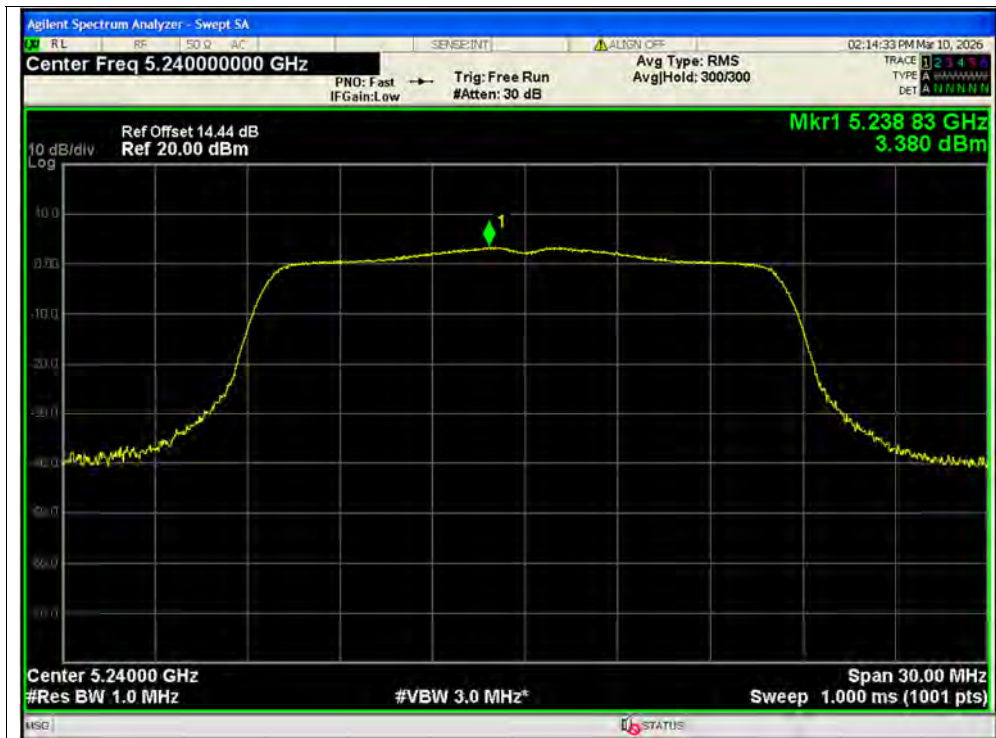
PSD NVNT a 5240MHz Ant2 SISO
