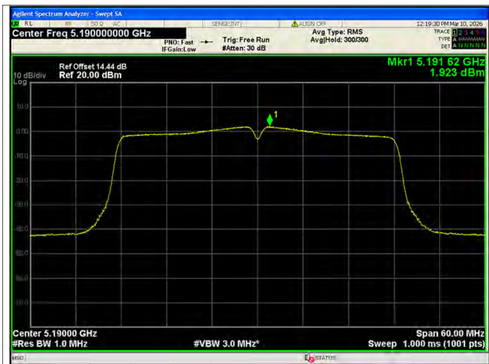
PSD NVNT n40 5190MHz Ant1 SISO
