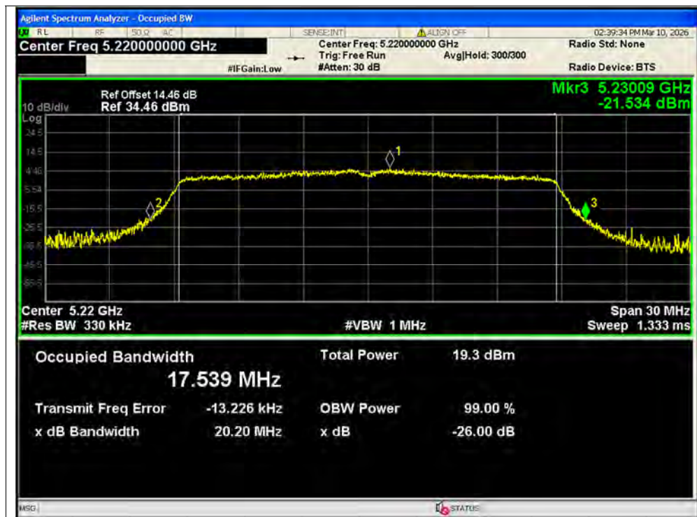
-26dB Bandwidth NVNT ac20 5220MHz Ant2 SISO
