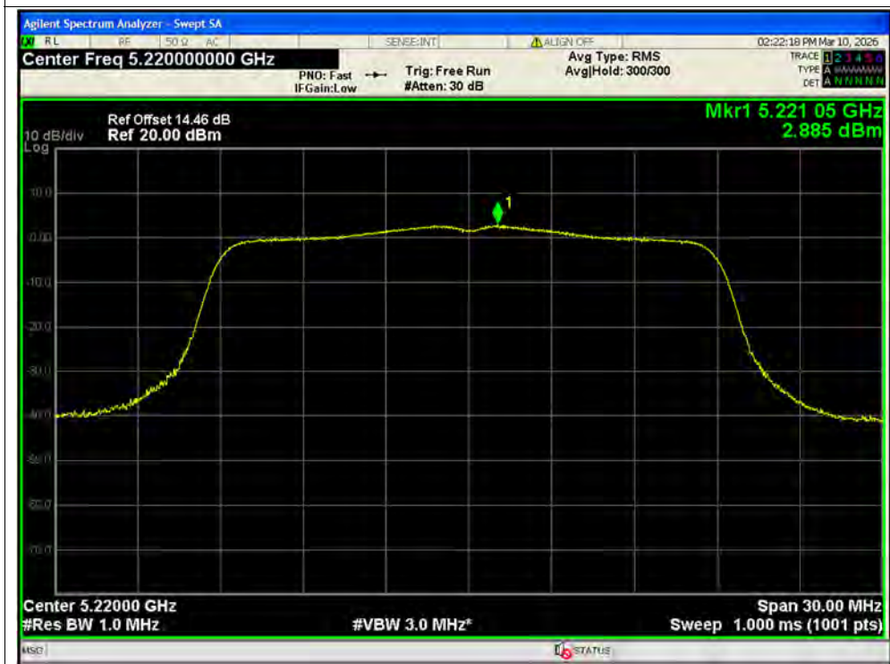
PSD NVNT n20 5220MHz Ant2 SISO
