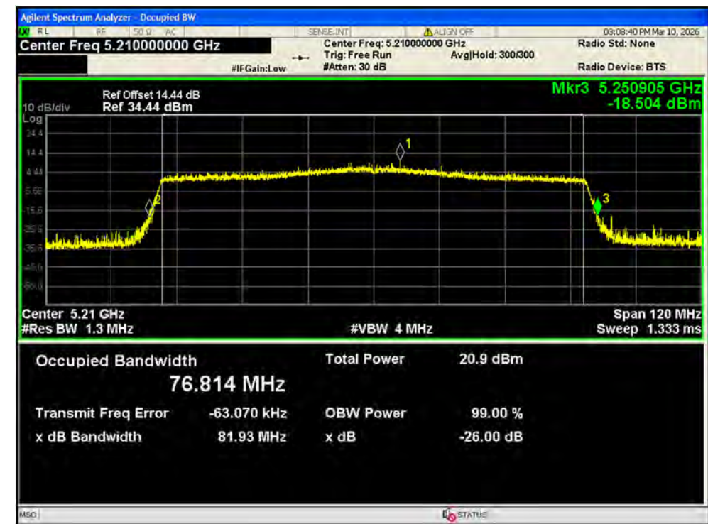
-26dB Bandwidth NVNT ax80 5210MHz Ant2 SISO
