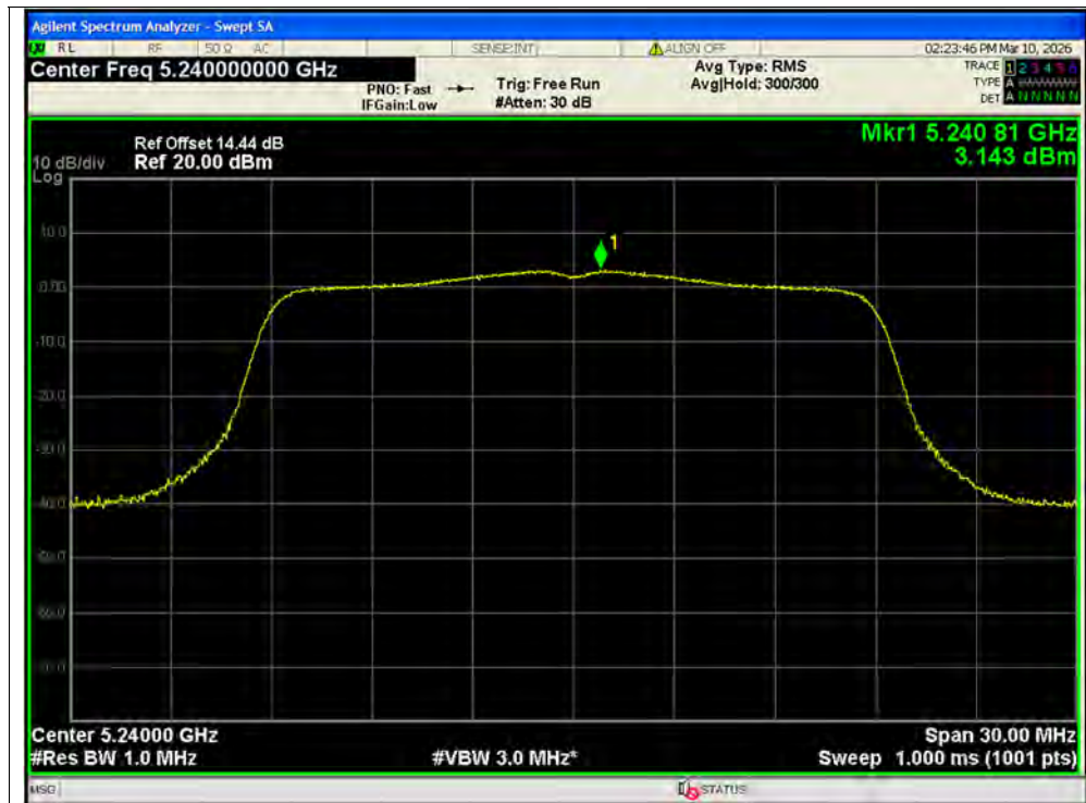
PSD NVNT n20 5240MHz Ant2 SISO
