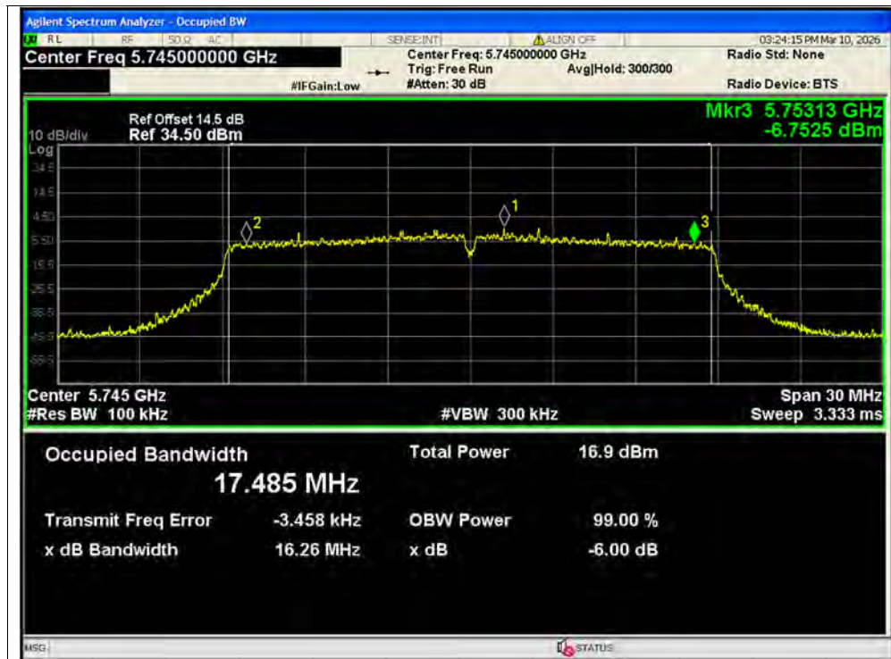
-6dB Bandwidth NVNT n20 5745MHz Ant1 MIMO
