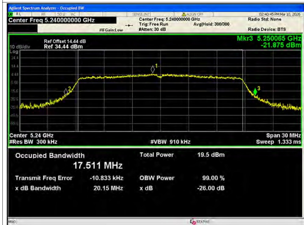
-26dB Bandwidth NVNT ac20 5240MHz Ant2 SISO
