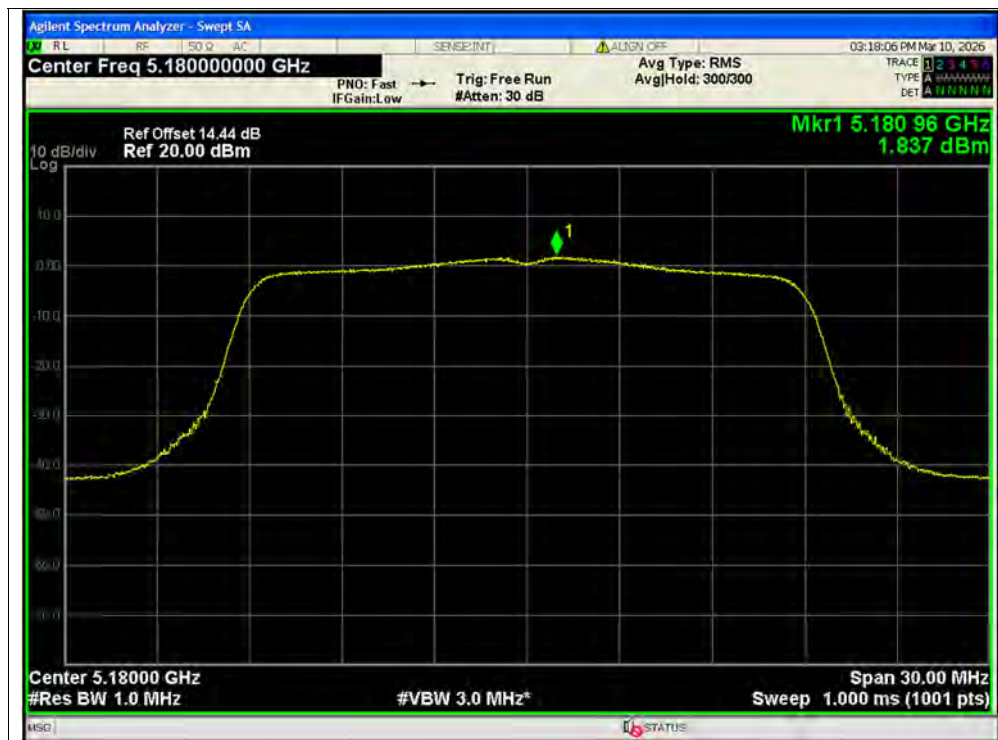
PSD NVNT n20 5180MHz Ant1 MIMO
