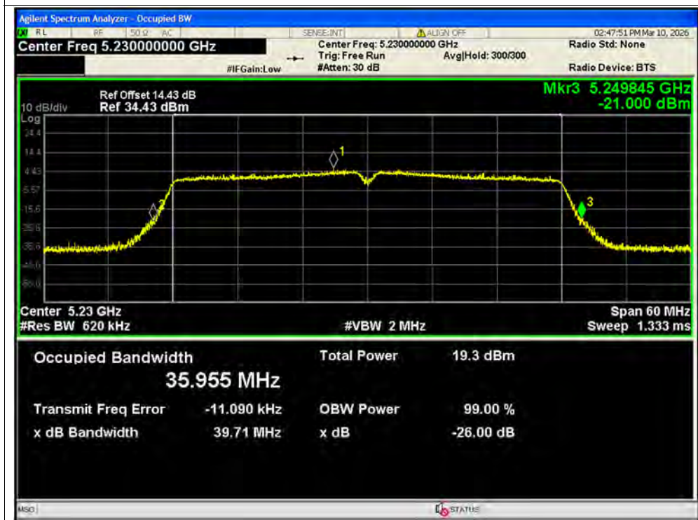
-26dB Bandwidth NVNT ac40 5230MHz Ant2 SISO
