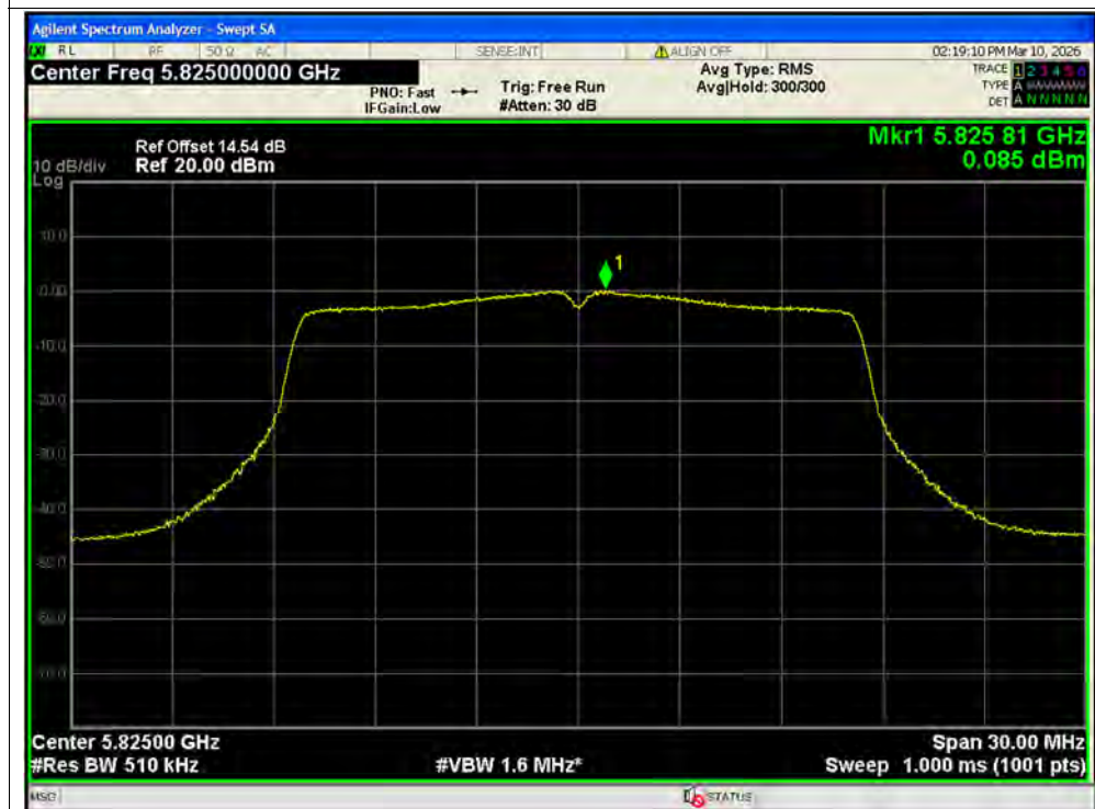
PSD NVNT a 5825MHz Ant2 SISO
