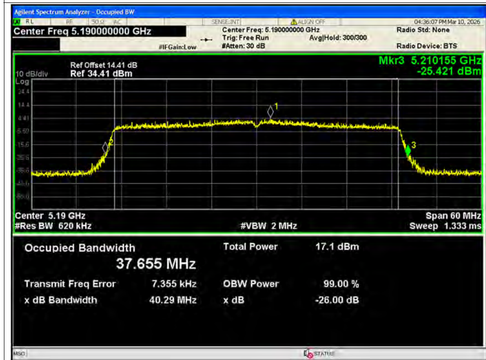
-26dB Bandwidth NVNT ax40 5190MHz Ant2 MIMO
