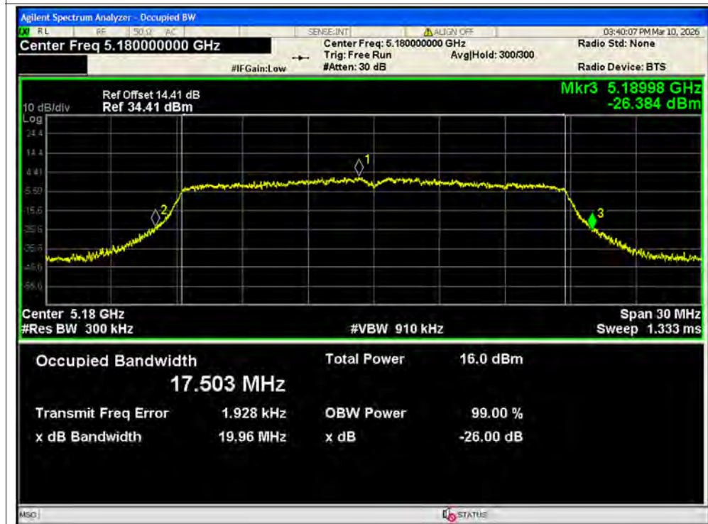
-26dB Bandwidth NVNT ac20 5180MHz Ant2 MIMO
