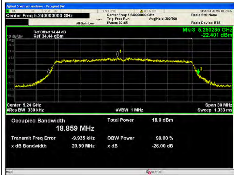
-26dB Bandwidth NVNT ax20 5240MHz Ant2 MIMO
