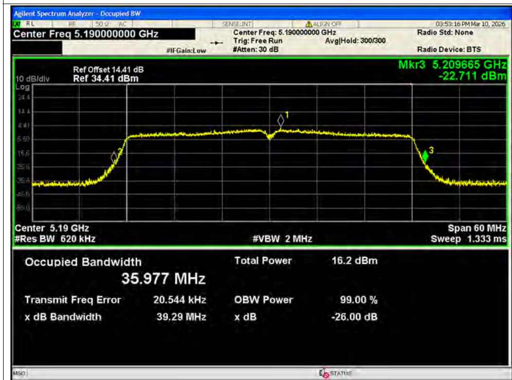
-26dB Bandwidth NVNT ac40 5190MHz Ant2 MIMO
