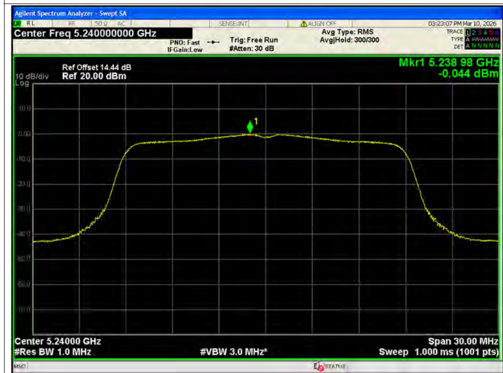
PSD NVNT n20 5240MHz Ant2 MIMO
