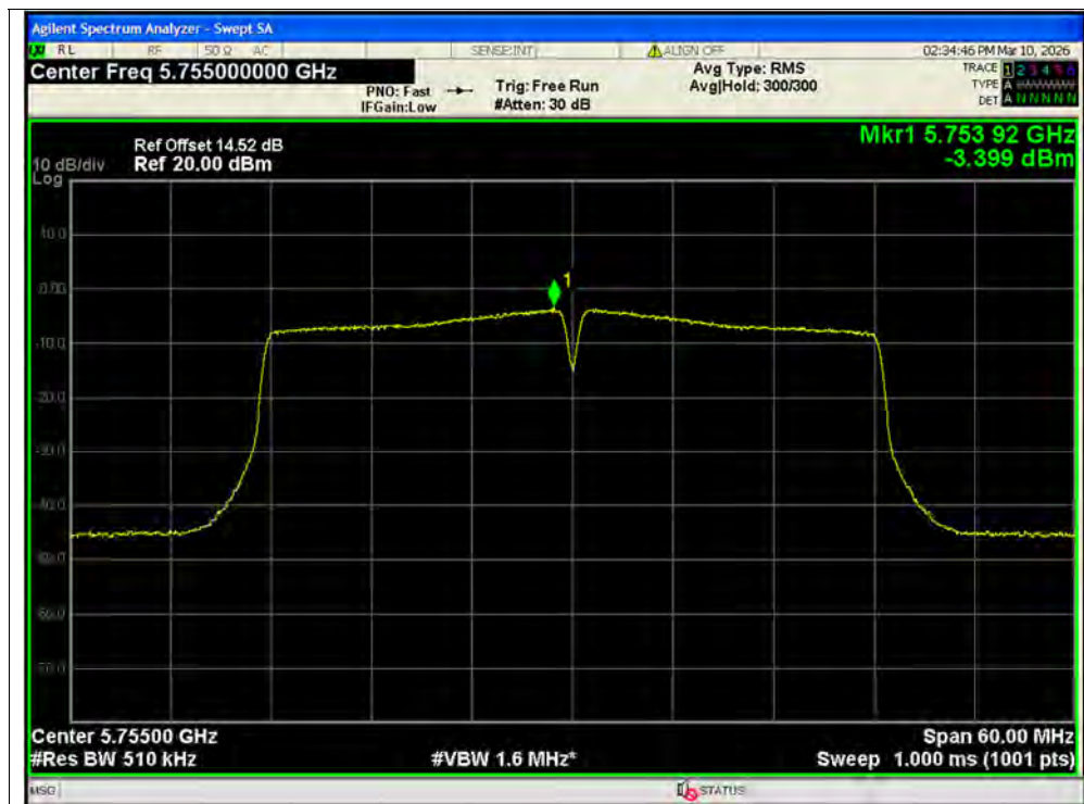
PSD NVNT n40 5755MHz Ant2 SISO
