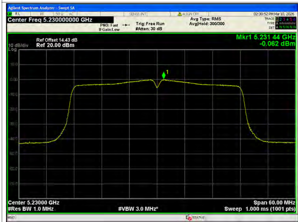
PSD NVNT n40 5230MHz Ant2 SISO
