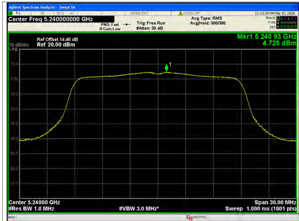
PSD NVNT n20 5240MHz Ant1 SISO
