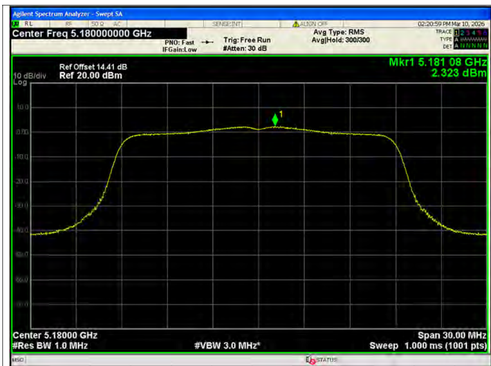
PSD NVNT n20 5180MHz Ant2 SISO
