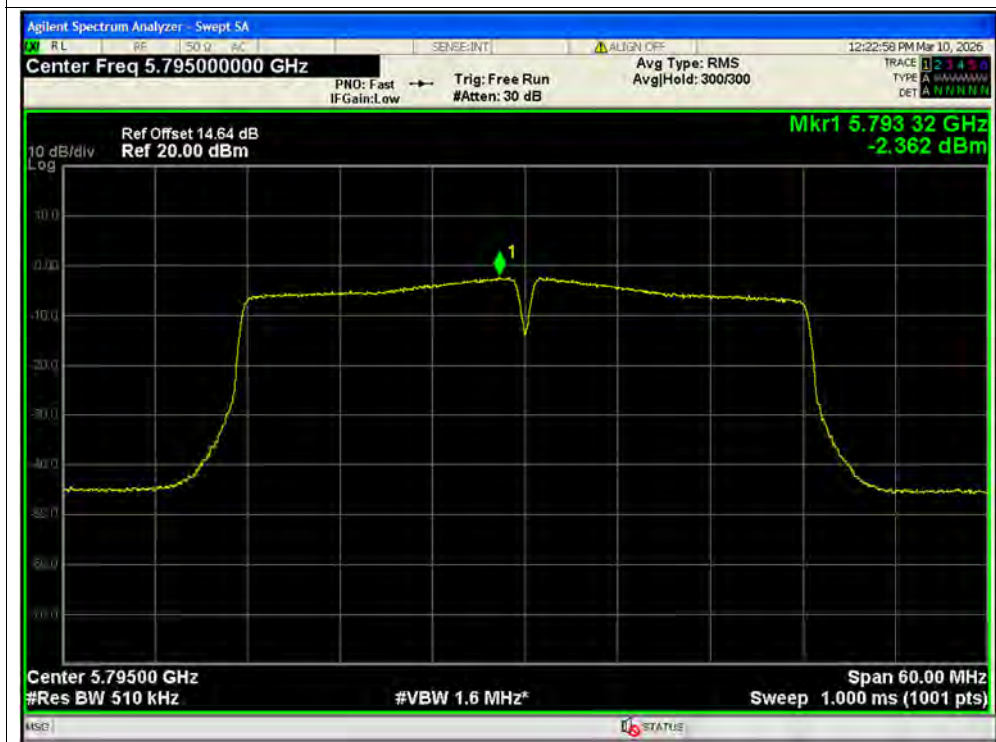
PSD NVNT n40 5795MHz Ant1 SISO
