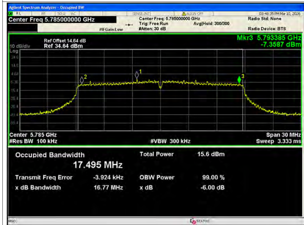
-6dB Bandwidth NVNT ac20 5785MHz Ant2 MIMO
