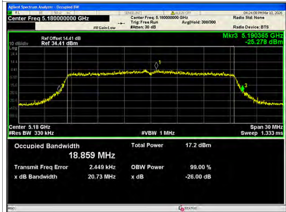
-26dB Bandwidth NVNT ax20 5180MHz Ant2 MIMO
