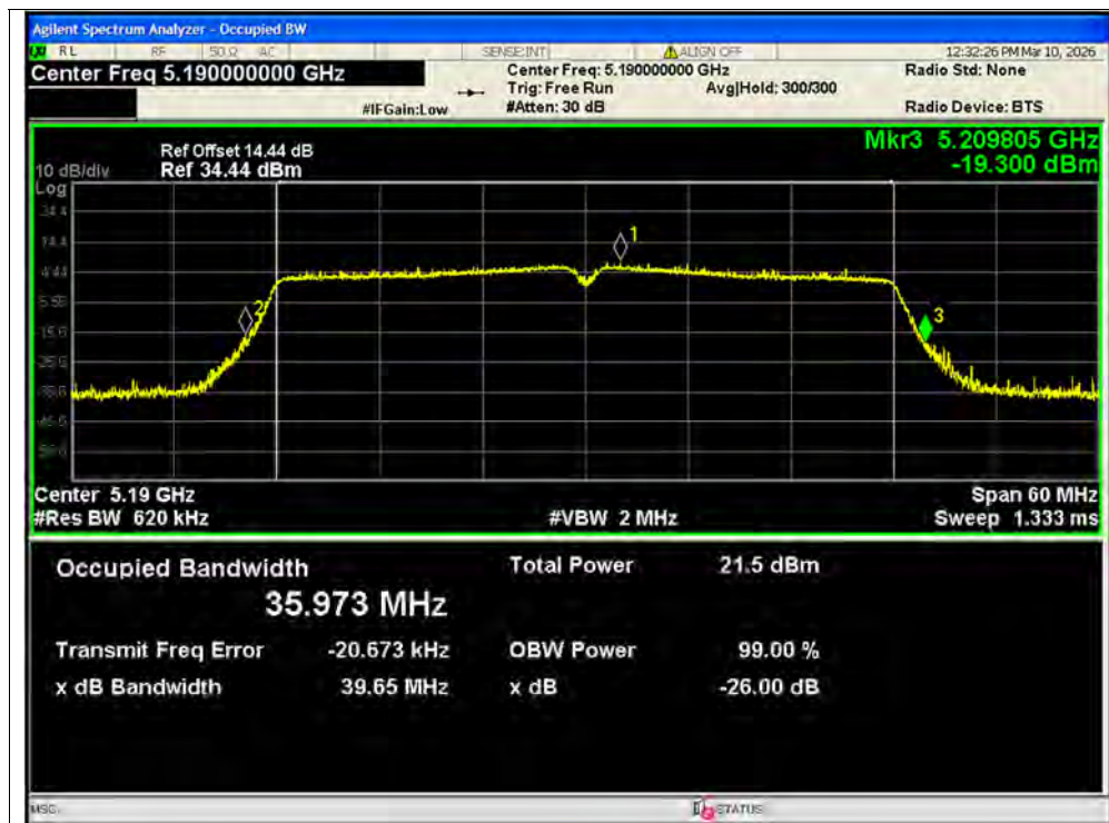
-26dB Bandwidth NVNT ac40 5190MHz Ant1 SISO
