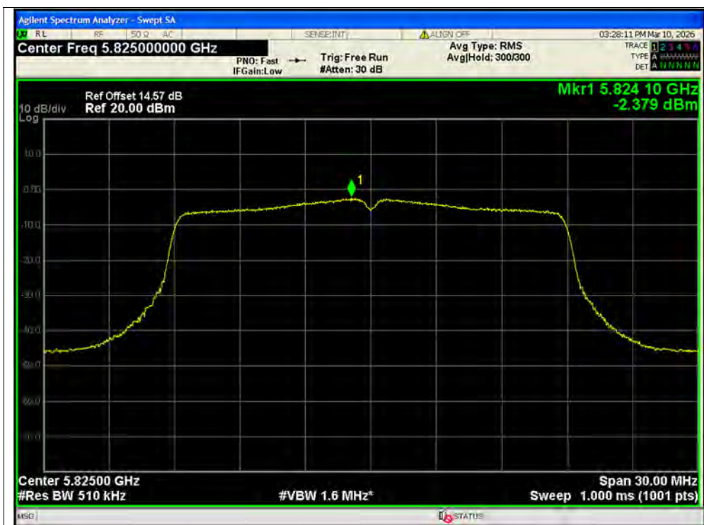
PSD NVNT n20 5825MHz Ant1 MIMO
