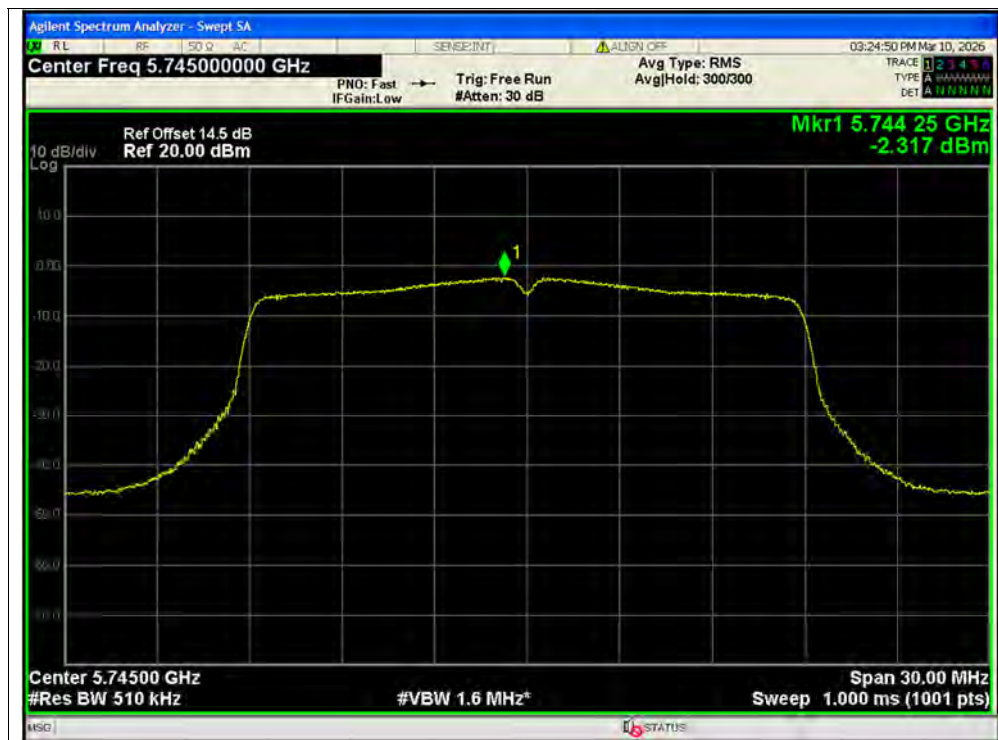
PSD NVNT n20 5745MHz Ant1 MIMO
