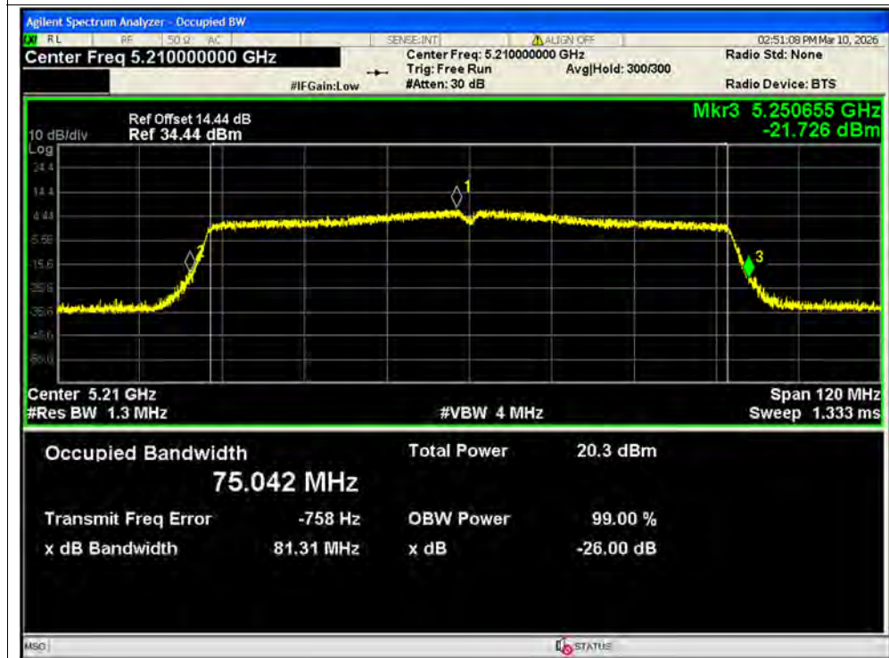
-26dB Bandwidth NVNT ac80 5210MHz Ant2 SISO
