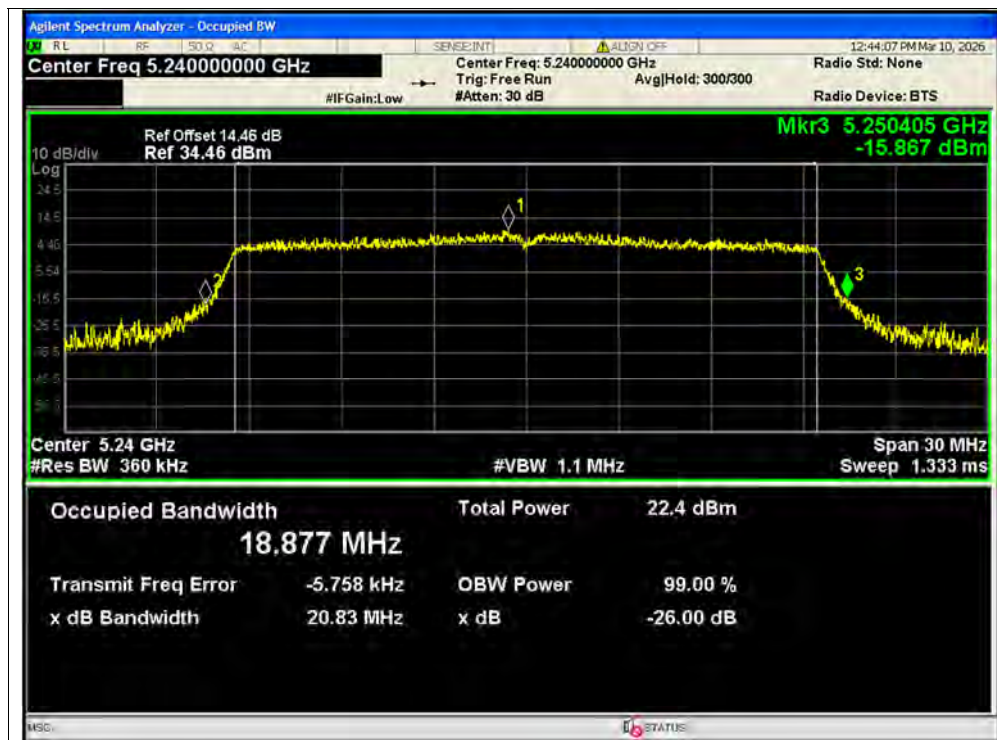
-26dB Bandwidth NVNT ax20 5240MHz Ant1 SISO
