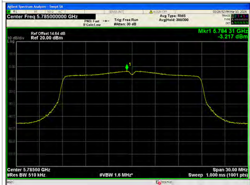
PSD NVNT n20 5785MHz Ant2 MIMO
