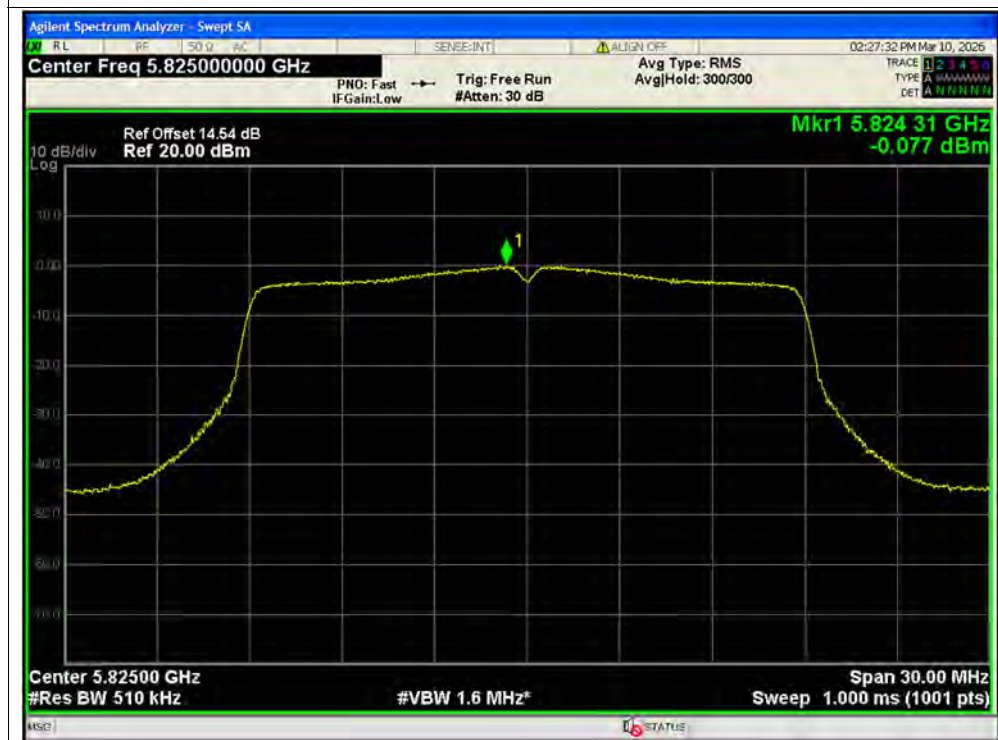
PSD NVNT n20 5825MHz Ant2 SISO
