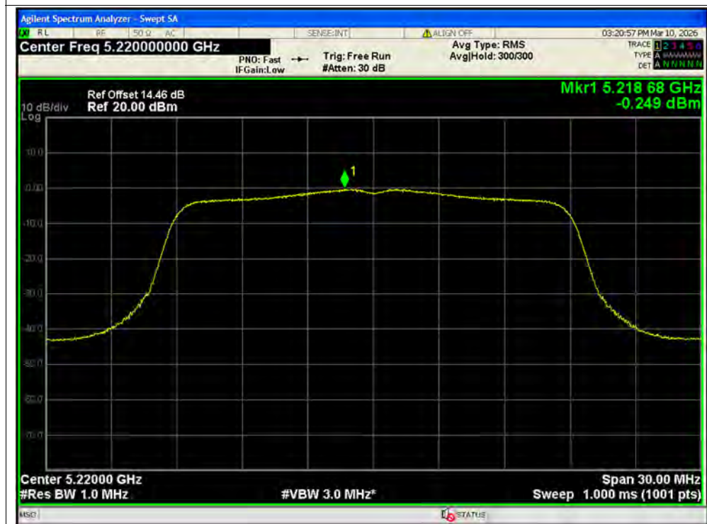
PSD NVNT n20 5220MHz Ant2 MIMO
