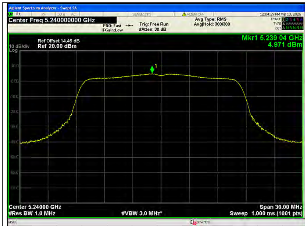
PSD NVNT a 5240MHz Ant1 SISO
