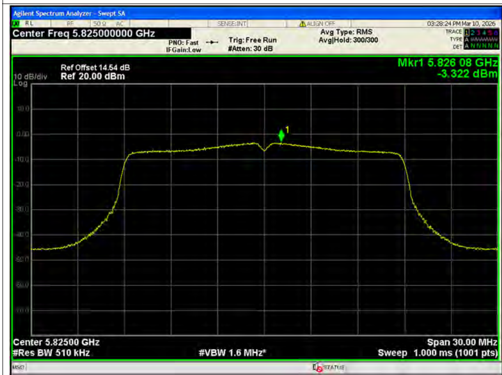
PSD NVNT n20 5825MHz Ant2 MIMO
