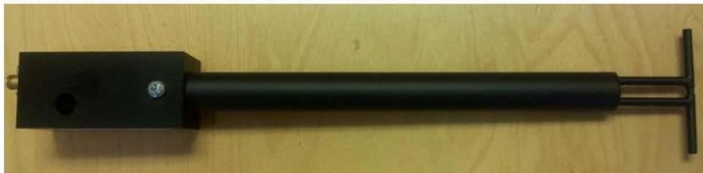
Figure 1 – MVG COMOSAR Validation Dipole
