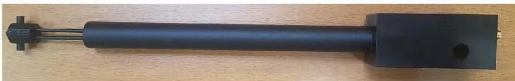
Figure 1 – MVG COMOSAR Validation Dipole
