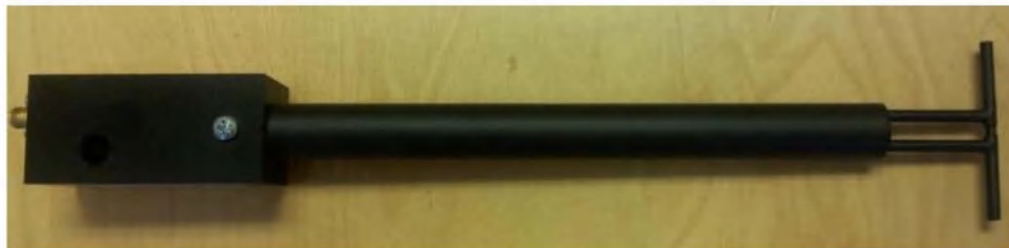
Figure 1 – MVG COMOSAR Validation Dipole
