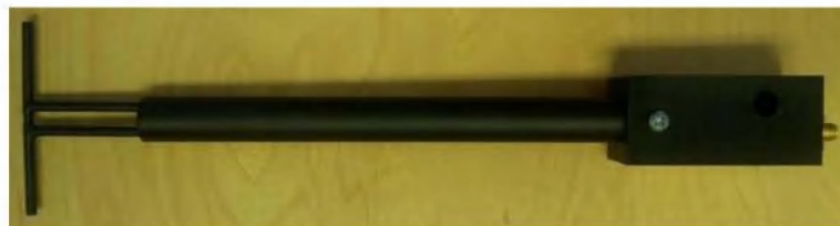
Figure 1 – MVG COMOSAR Validation Dipole
