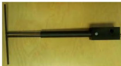
Figure 1 – MVG COMOSAR Validation Dipole
