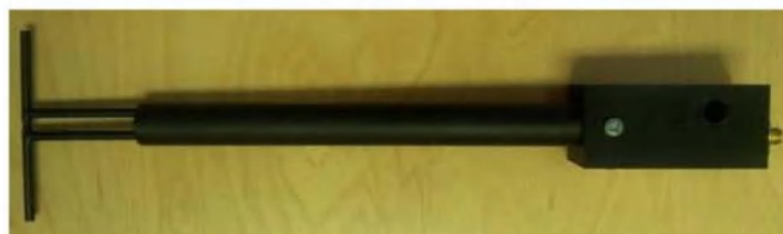
Figure 1 – MVG COMOSAR Validation Dipole
