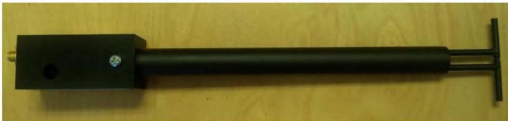
Figure 1 – MVG COMOSAR Validation Dipole
