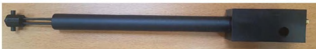
Figure 1 – MVG COMOSAR Validation Dipole
