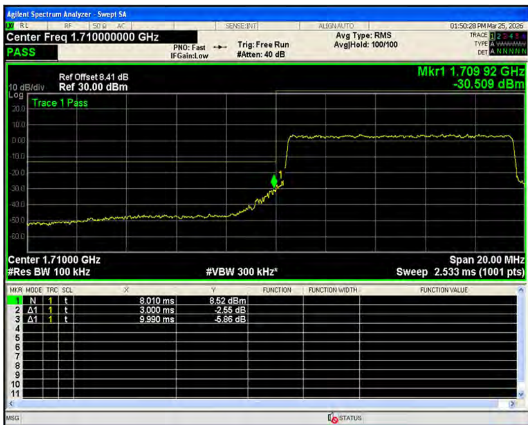
Band66 QPSK BW=10MHz Channel=132622 RB Size=50 Position=#0
