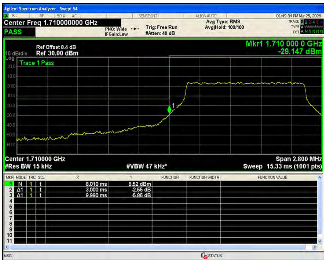
Band66 QPSK BW=1.4MHz Channel=132665 RB Size=6 Position=#0
