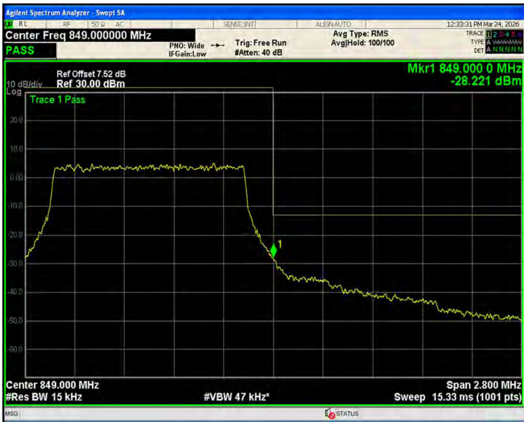
Band5 QPSK BW=3MHz Channel=20415 RB Size=15 Position=#0
