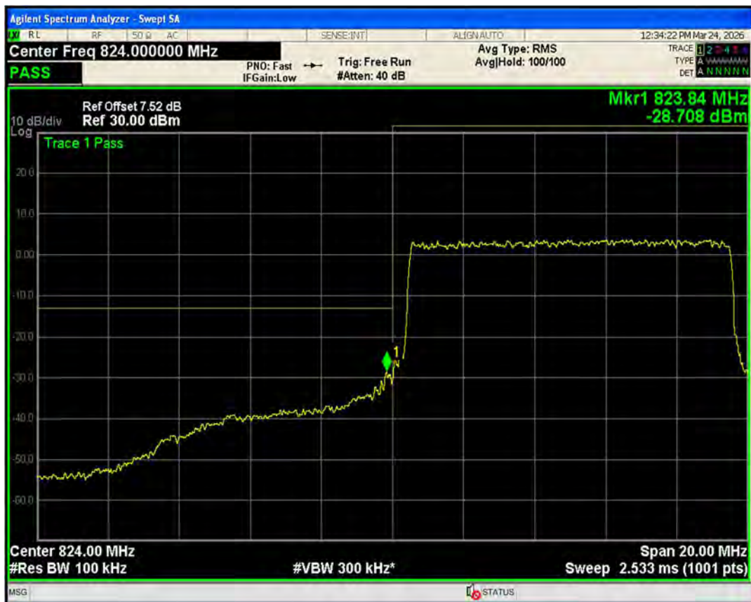
Band5 QPSK BW=10MHz Channel=20600 RB Size=50 Position=#0
