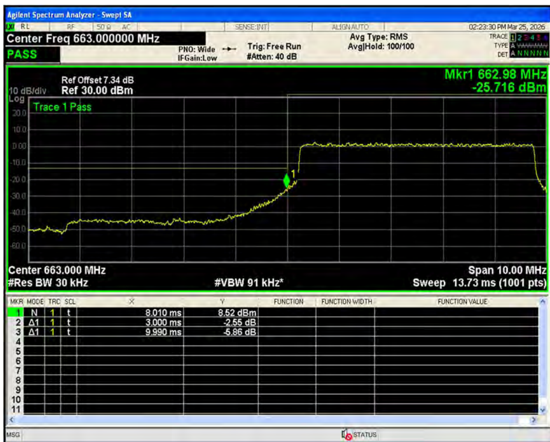
Band71 QPSK BW=5MHz Channel=133447 RB Size=25 Position=#0
