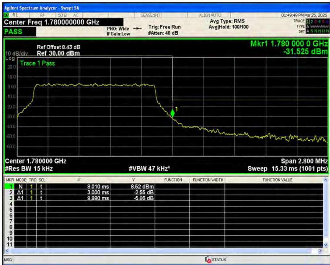
Band66 16QAM BW=3MHz Channel=131987 RB Size=15 Position=#0
