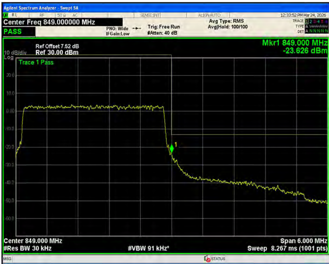
Band5 QPSK BW=5MHz Channel=20425 RB Size=25 Position=#0
