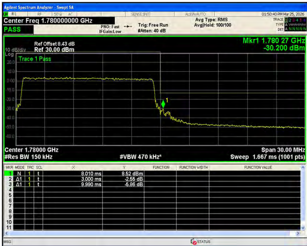
Band66 QPSK BW=20MHz Channel=132072 RB Size=100 Position=#0
