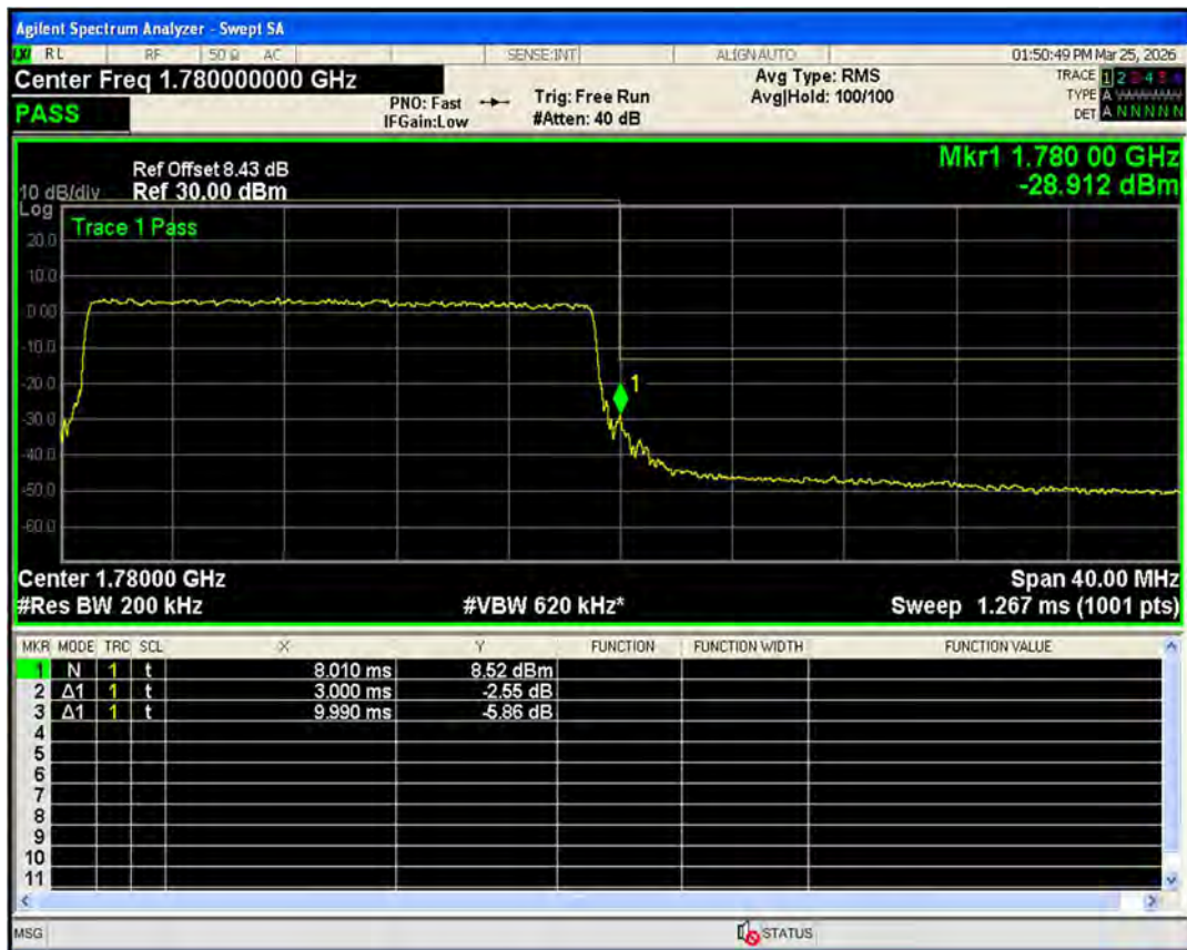
Band71 16QAM BW=5MHz Channel=133147 RB Size=25 Position=#0
