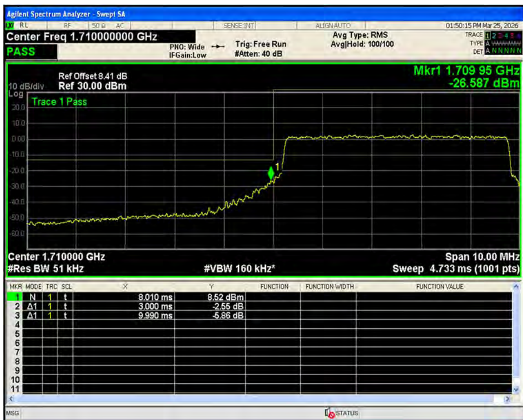
Band66 16QAM BW=5MHz Channel=132647 RB Size=25 Position=#0
