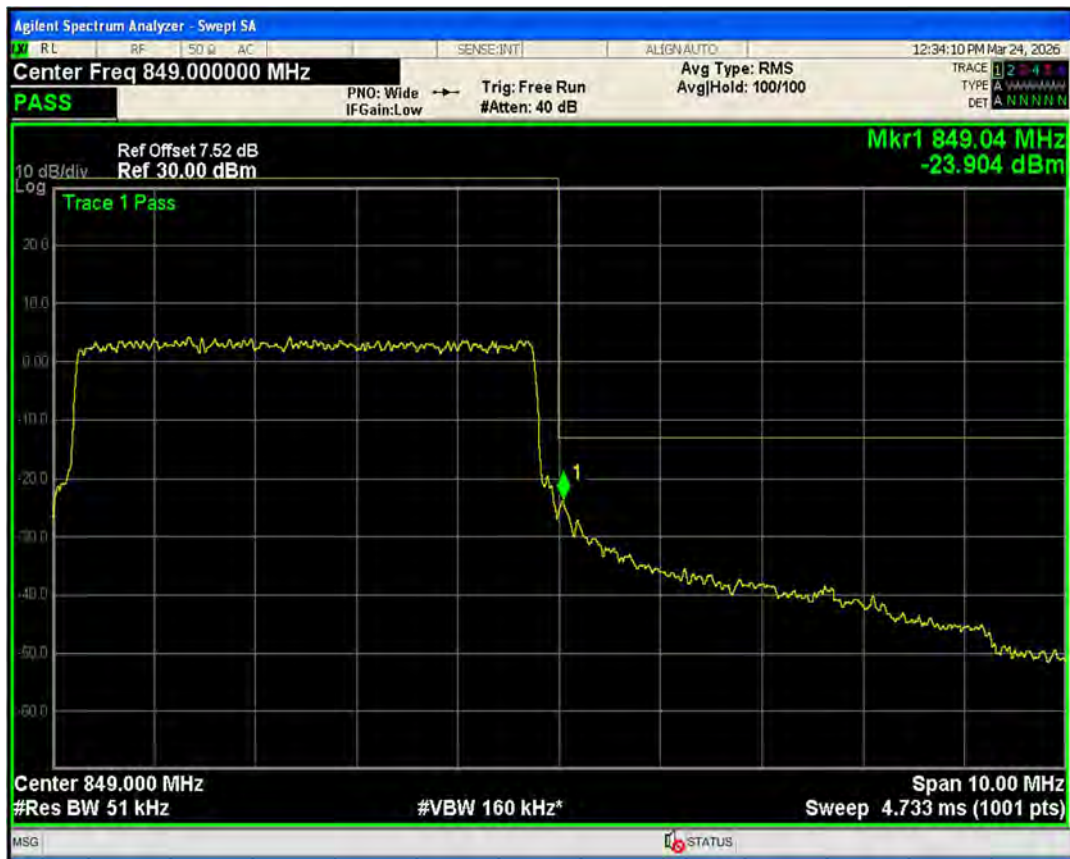
Band5 QPSK BW=10MHz Channel=20450 RB Size=50 Position=#0
