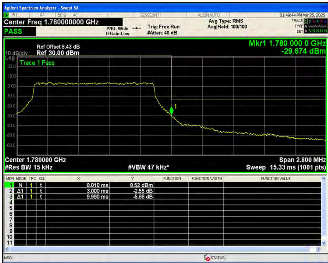
Band66 QPSK BW=3MHz Channel=131987 RB Size=15 Position=#0
