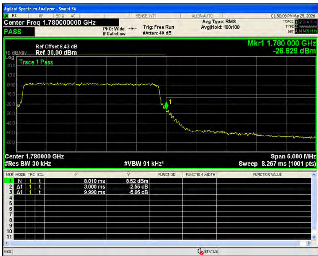
Band66 16QAM BW=5MHz Channel=131997 RB Size=25 Position=#0
