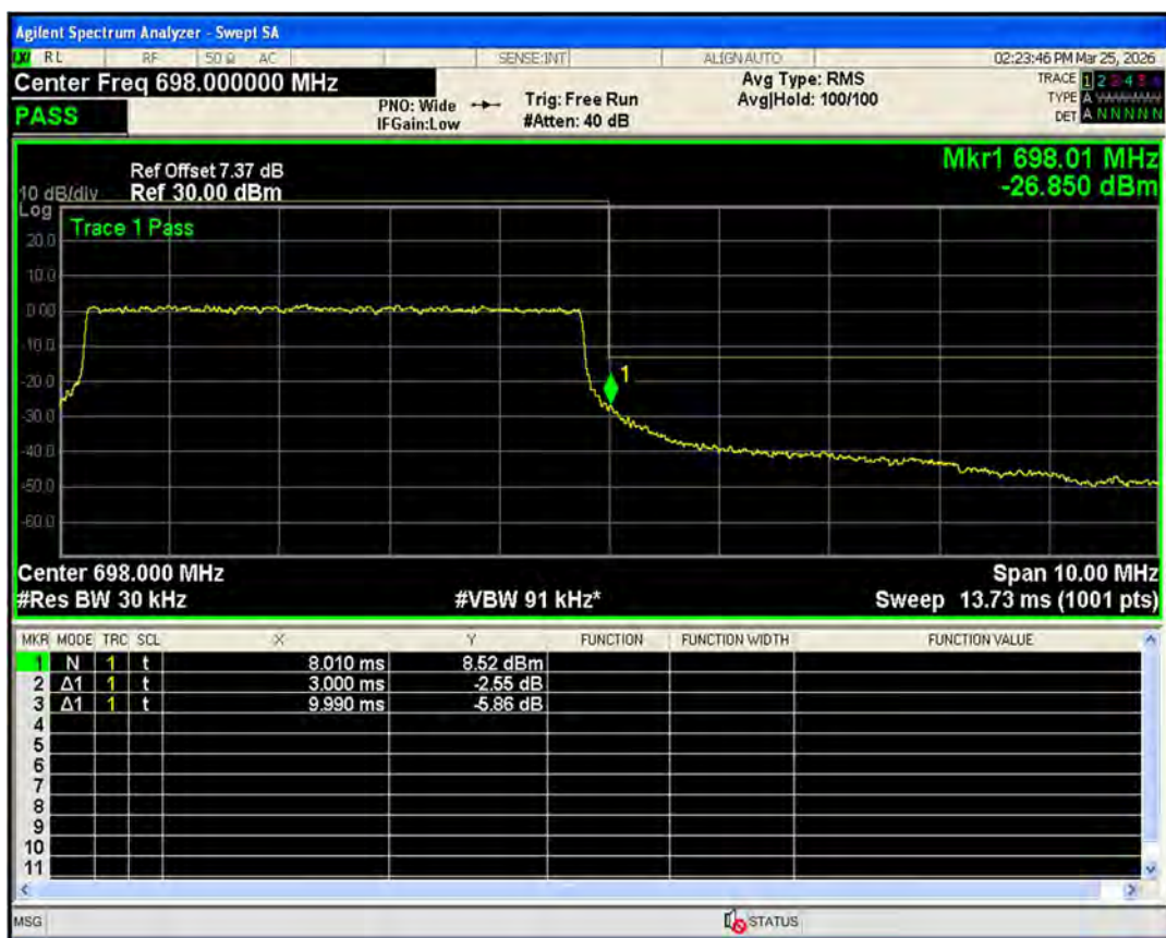
Band71 QPSK BW=5MHz Channel=133147 RB Size=25 Position=#0
