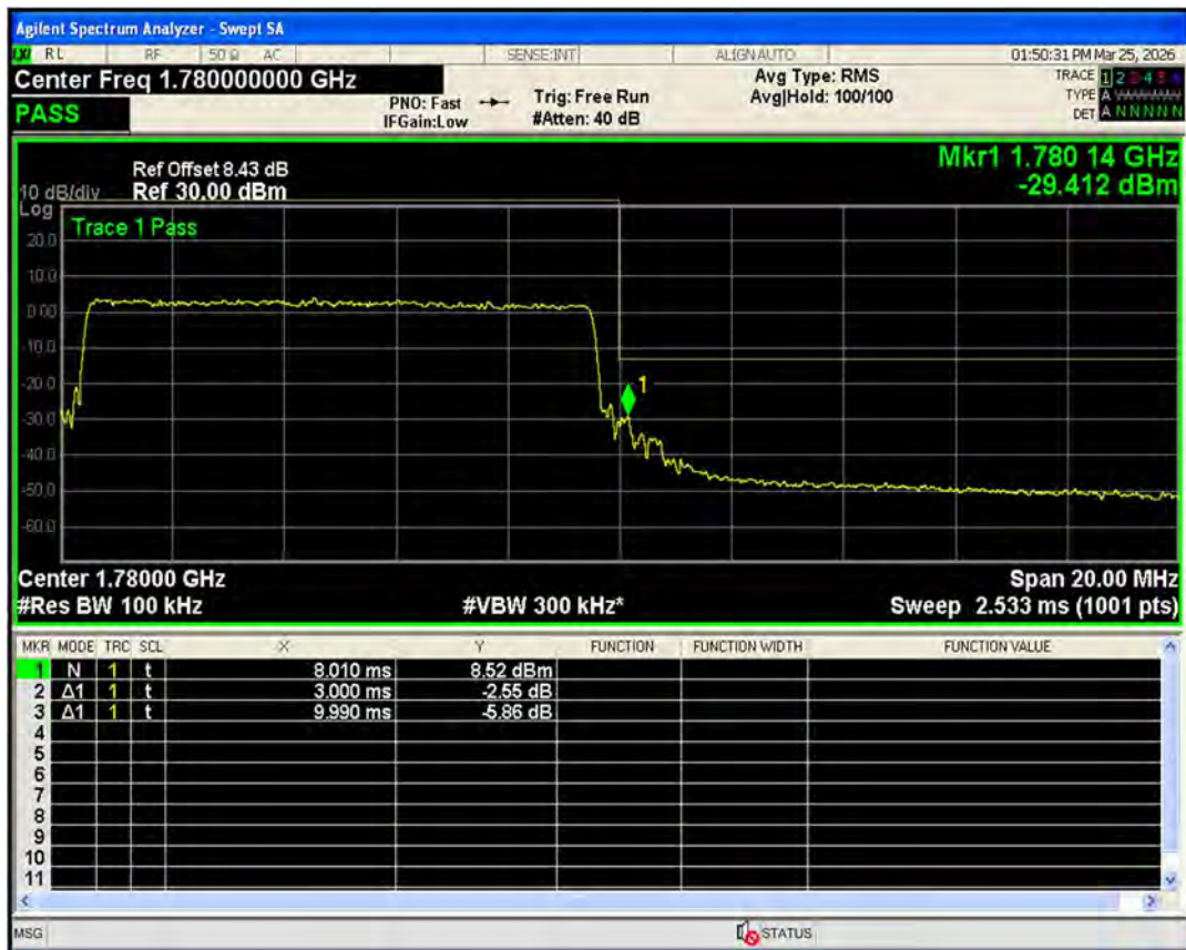
Band66 QPSK BW=15MHz Channel=132047 RB Size=75 Position=#0
