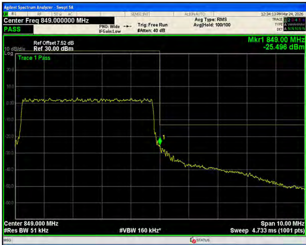
Band5 QPSK BW=1.4MHz Channel=20407 RB Size=6 Position=#0
