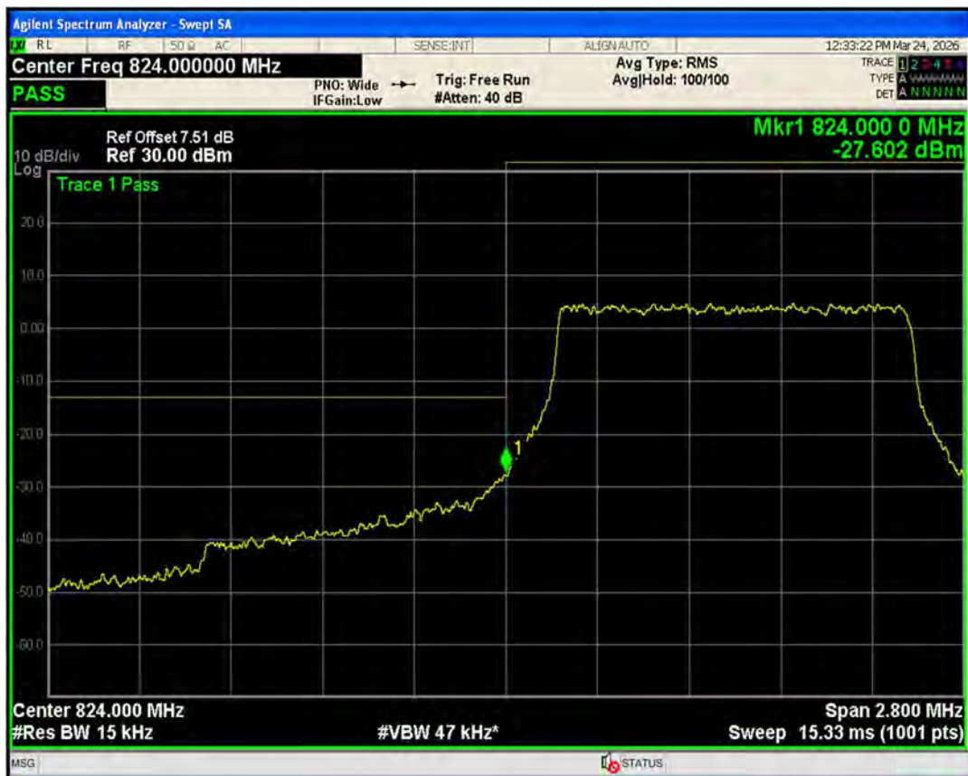
Band5 QPSK BW=1.4MHz Channel=20643 RB Size=6 Position=#0
