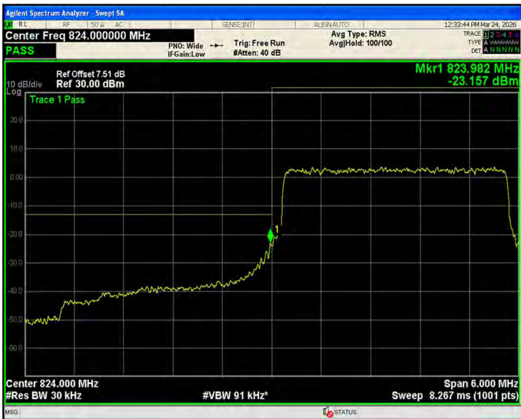
Band5 QPSK BW=3MHz Channel=20635 RB Size=15 Position=#0
