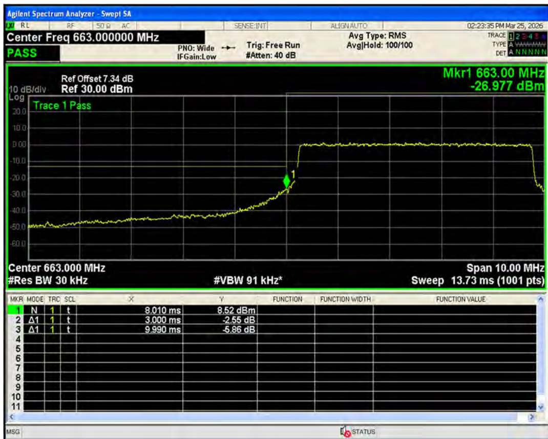
Band71 16QAM BW=5MHz Channel=133447 RB Size=25 Position=#0
