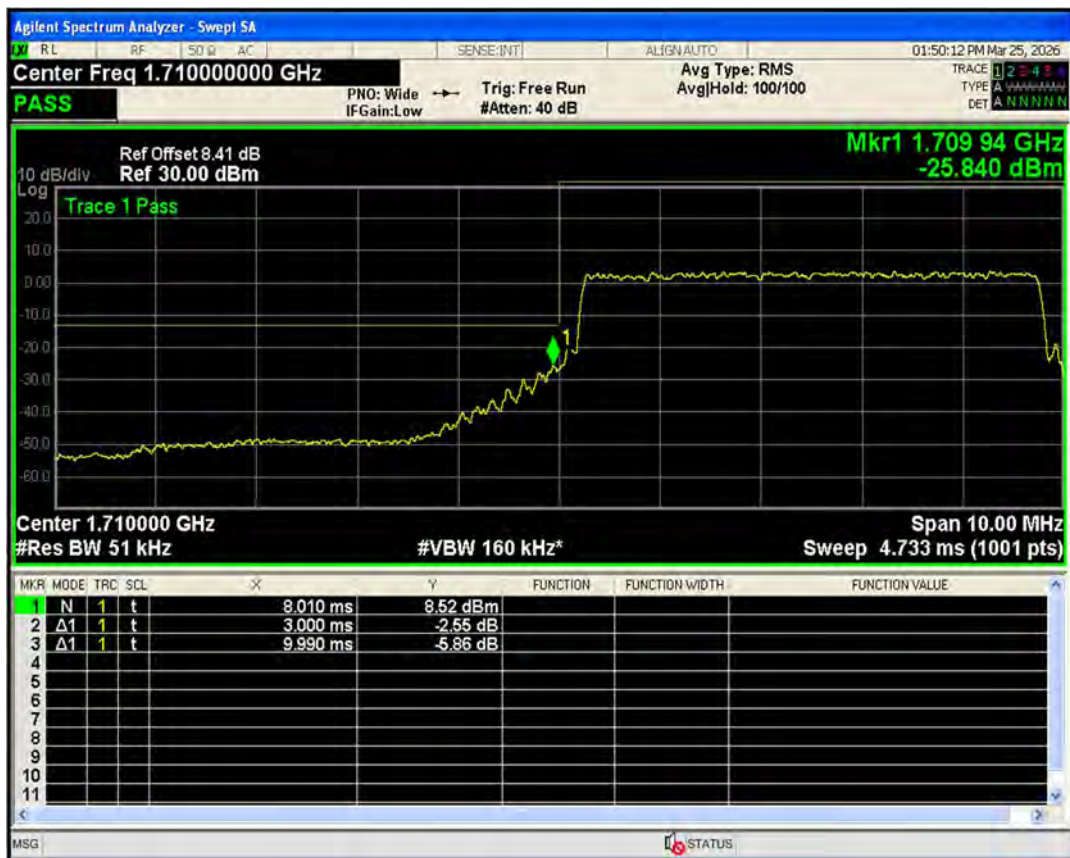
Band66 QPSK BW=5MHz Channel=132647 RB Size=25 Position=#0
