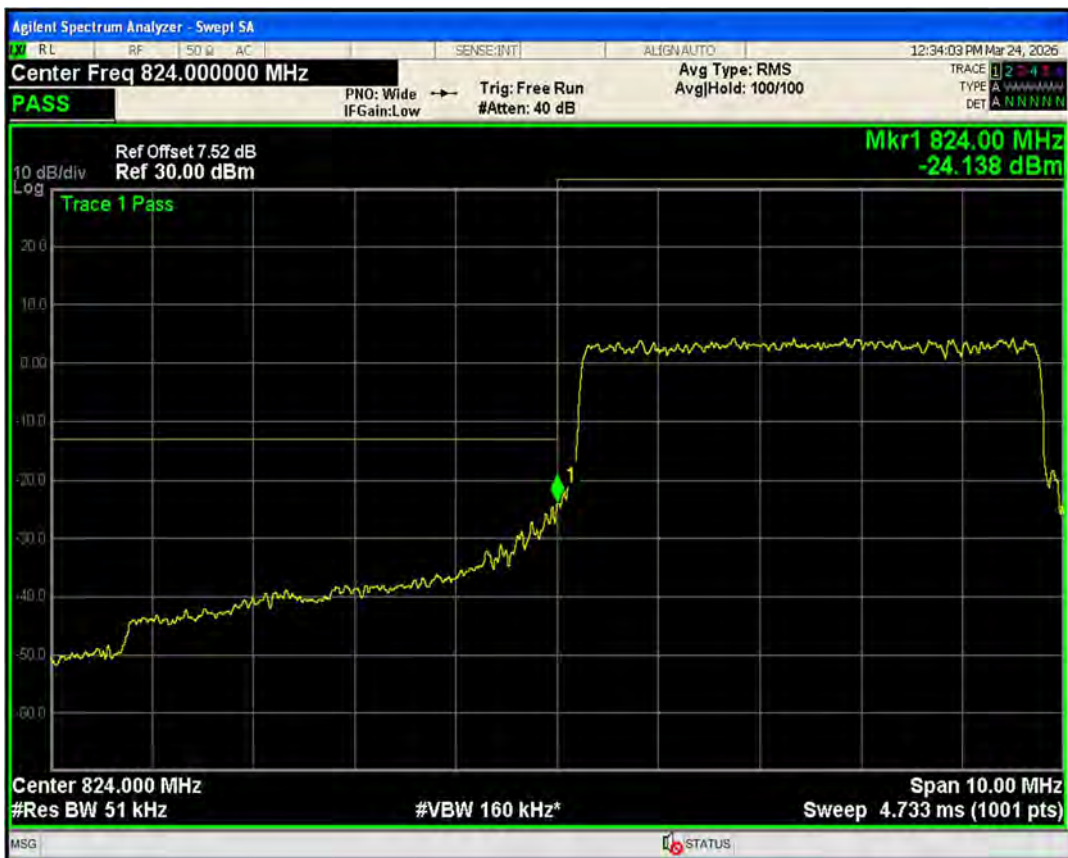
Band5 QPSK BW=5MHz Channel=20625 RB Size=25 Position=#0
