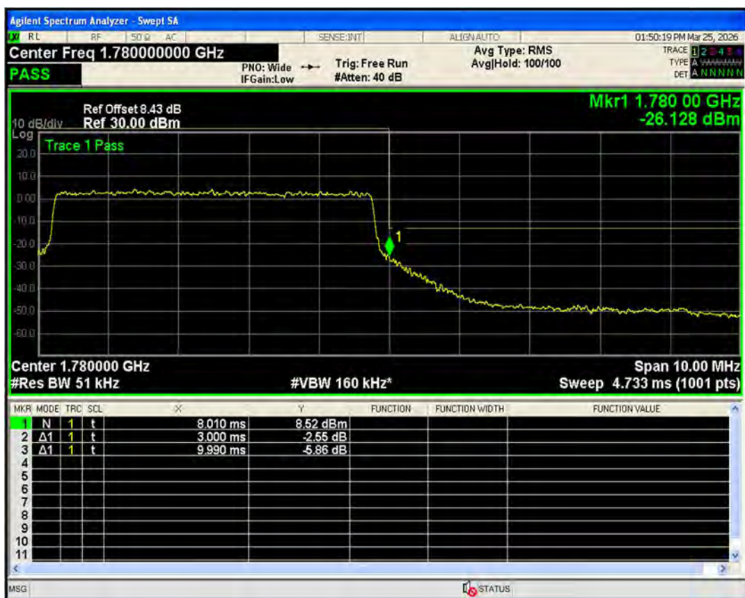
Band66 QPSK BW=10MHz Channel=132022 RB Size=50 Position=#0
