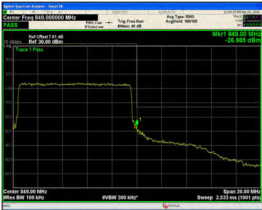
Band66 16QAM BW=1.4MHz Channel=131979 RB Size=6 Position=#0
