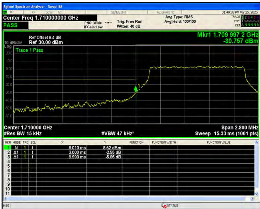
Band66 16QAM BW=1.4MHz Channel=132665 RB Size=6 Position=#0
