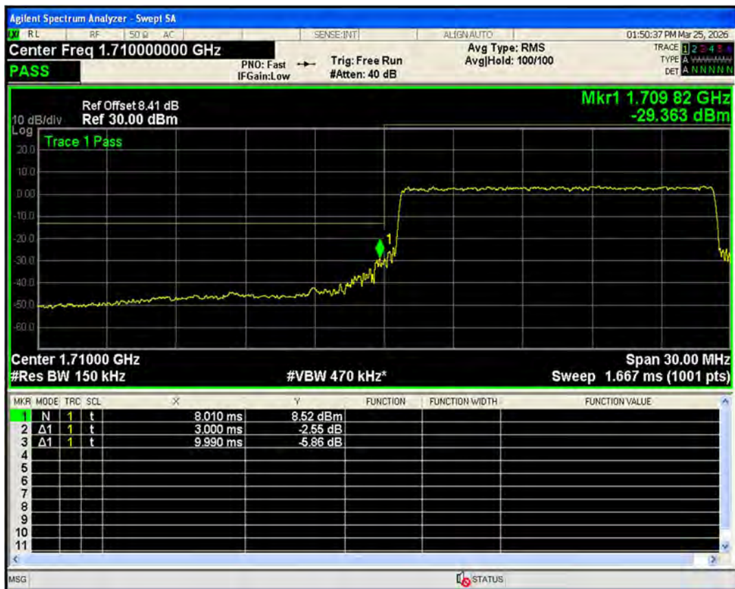
Band66 QPSK BW=15MHz Channel=132597 RB Size=75 Position=#0
