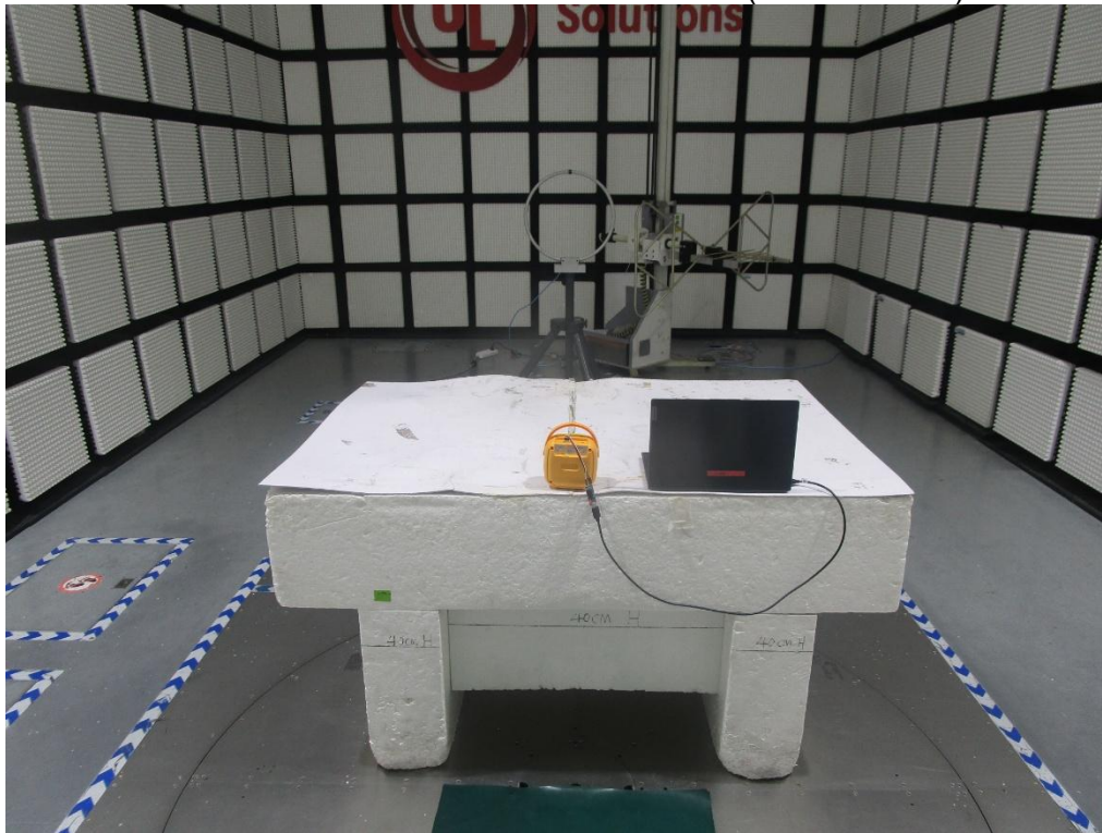
RADIATED RF MEASUREMENT SETUP (Below 30MHz)
