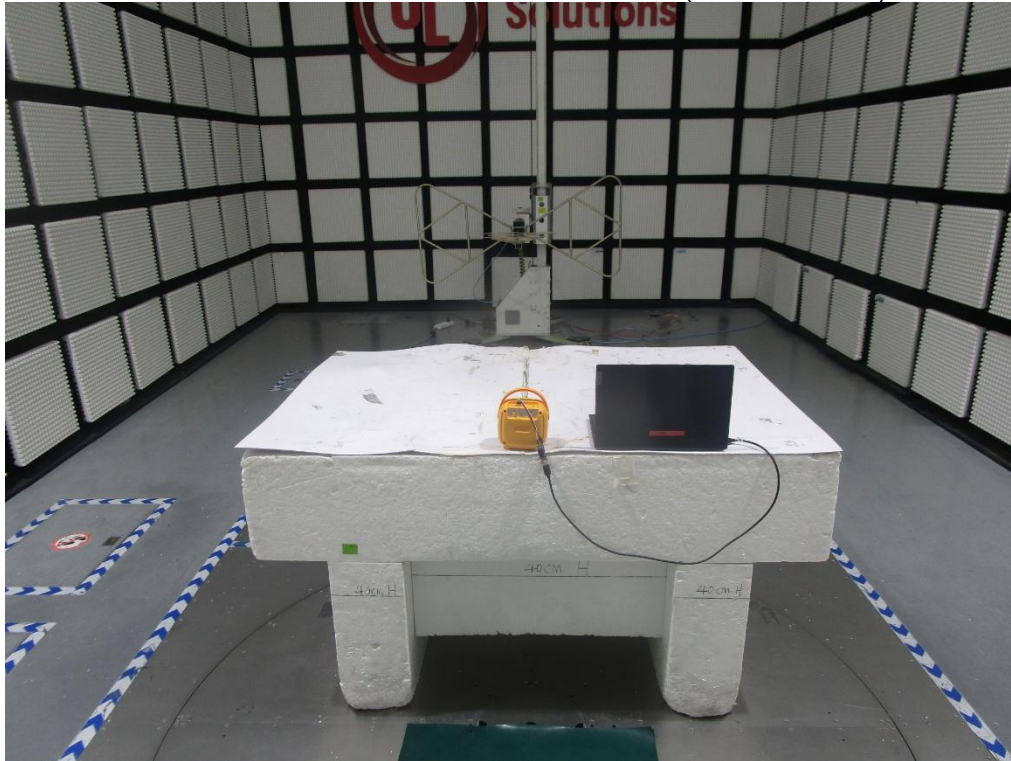
RADIATED RF MEASUREMENT SETUP (Below 30MHz)
