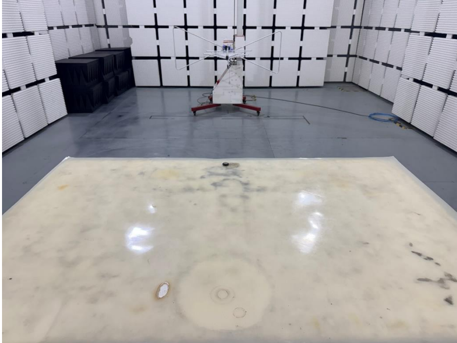
Set-up for Radiated Spurious Emission, Above 1GHz
