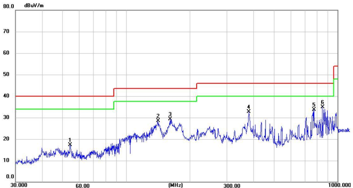
Radiated Emission Measurement
