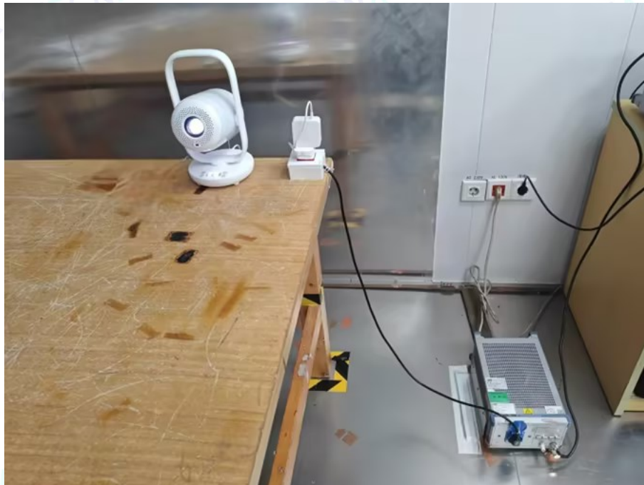
Photo of Setup for Radiated Emission (30MHz~1GHz)
