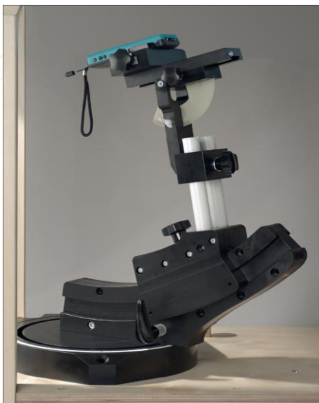
F-2. Device Holder for Transmitters
