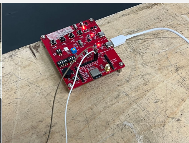
AC conducted test close-up
