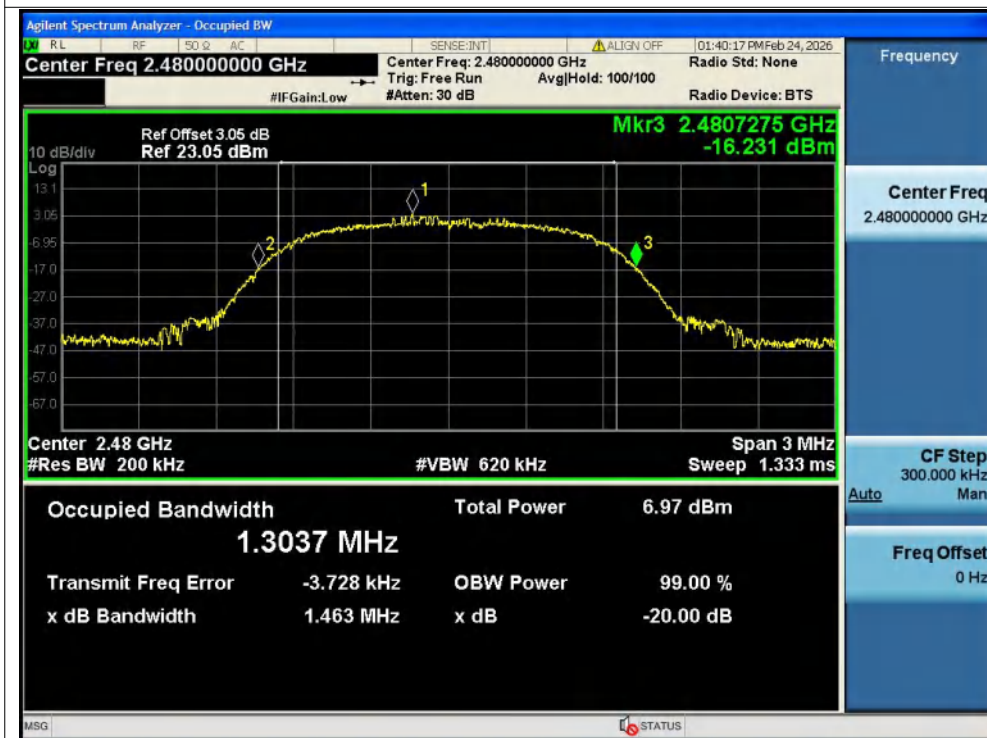
-20dB Bandwidth NVNT 2-DH5 2480MHz Ant1
