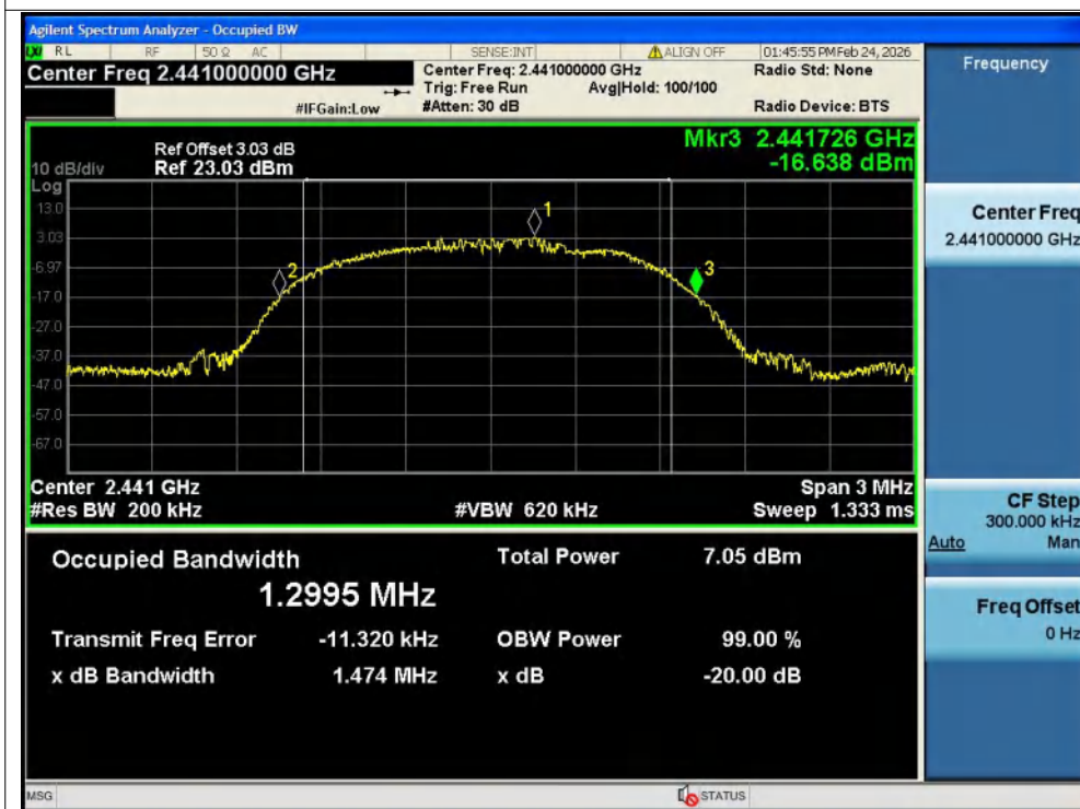
-20dB Bandwidth NVNT 3-DH5 2441MHz Ant1
