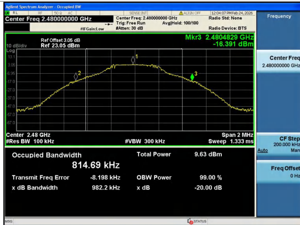
-20dB Bandwidth NVNT 2-DH5 2402MHz Ant1
