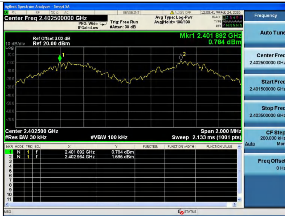
CFS NVNT 2-DH5 2402MHz Ant1
