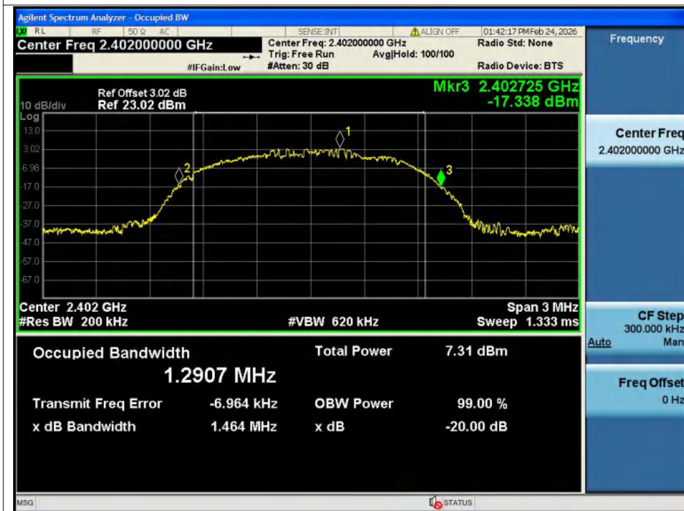
-20dB Bandwidth NVNT 3-DH5 2441MHz Ant1
