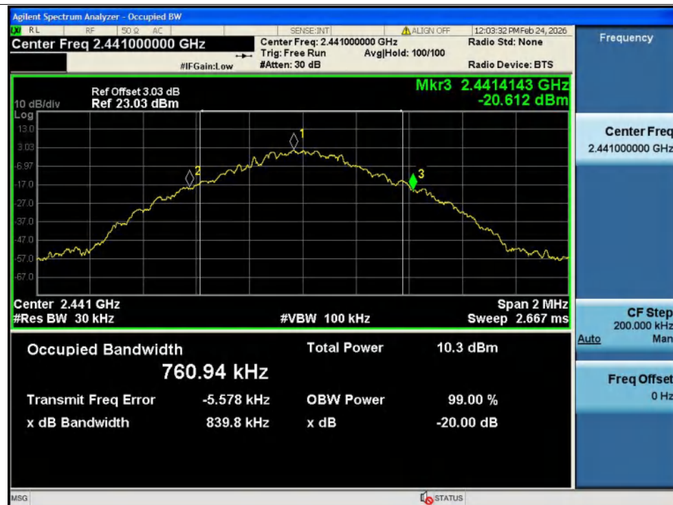
-20dB Bandwidth NVNT 1-DH5 2441MHz Ant1
