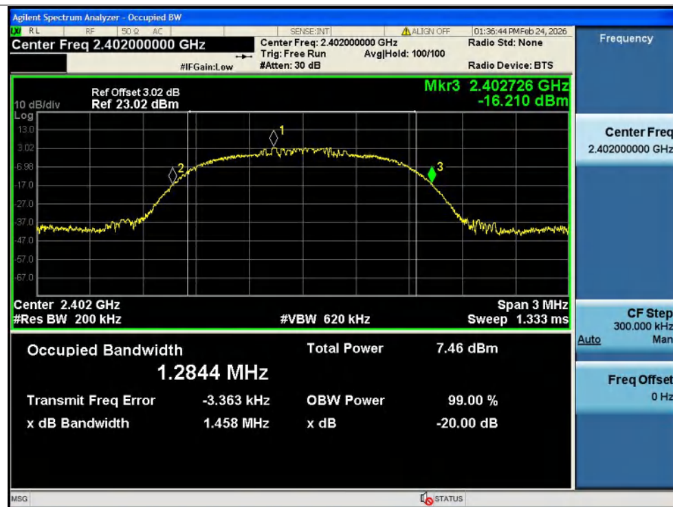
-20dB Bandwidth NVNT 2-DH5 2402MHz Ant1
