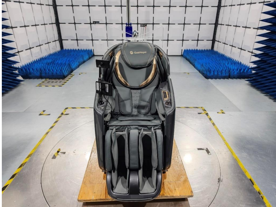
Radiated Emission Test Setup (Below 1GHz)
