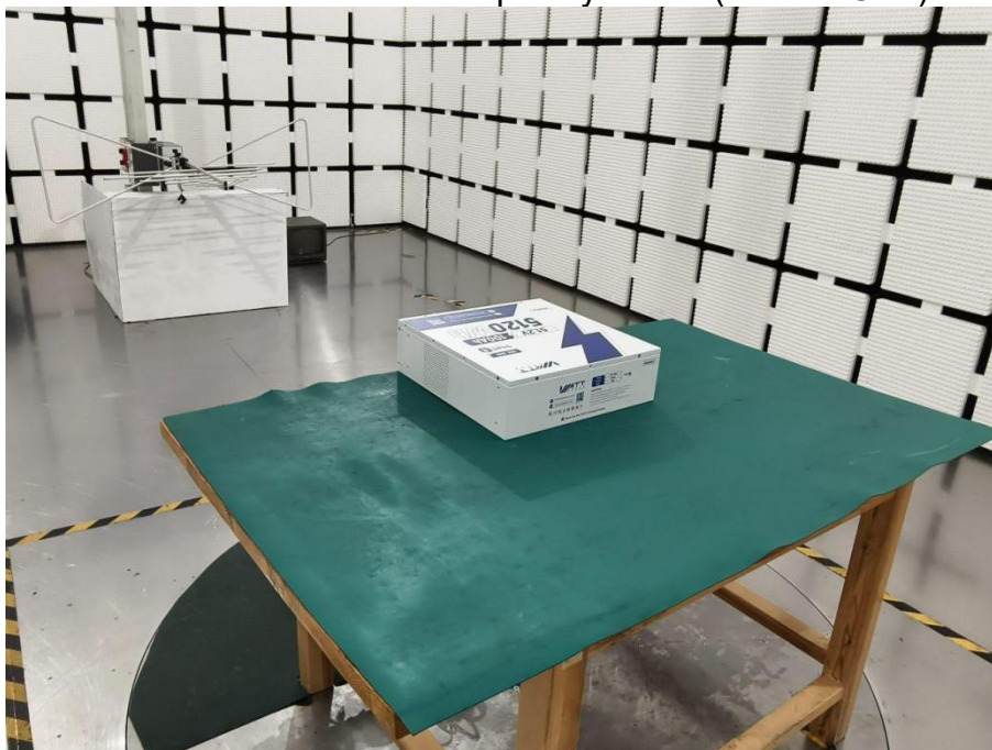
Emissions in restricted frequency bands (below 1GHz)
