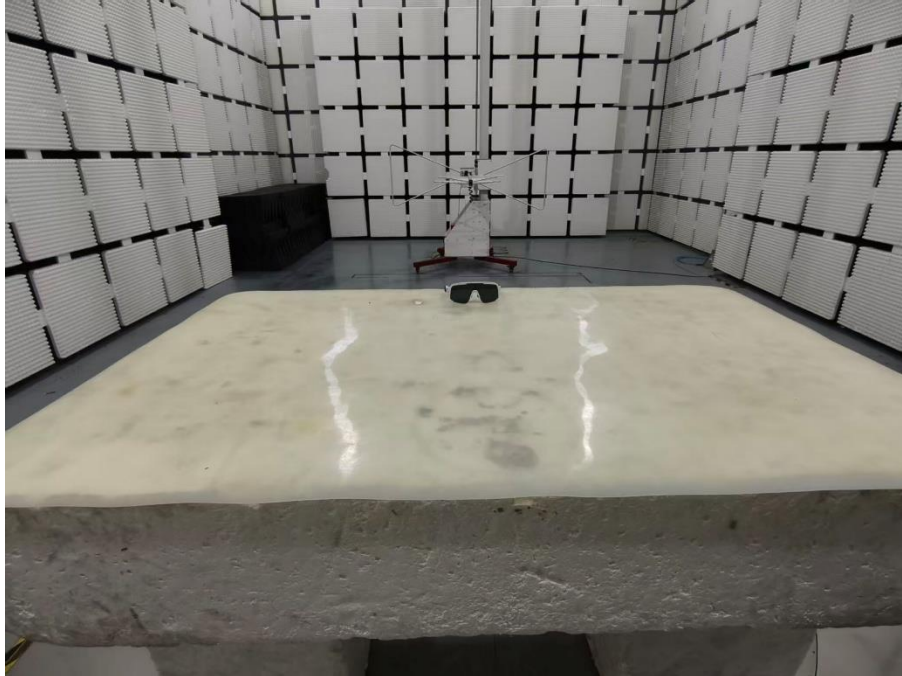
Set-up for Radiated Spurious Emission, Above 1GHz
