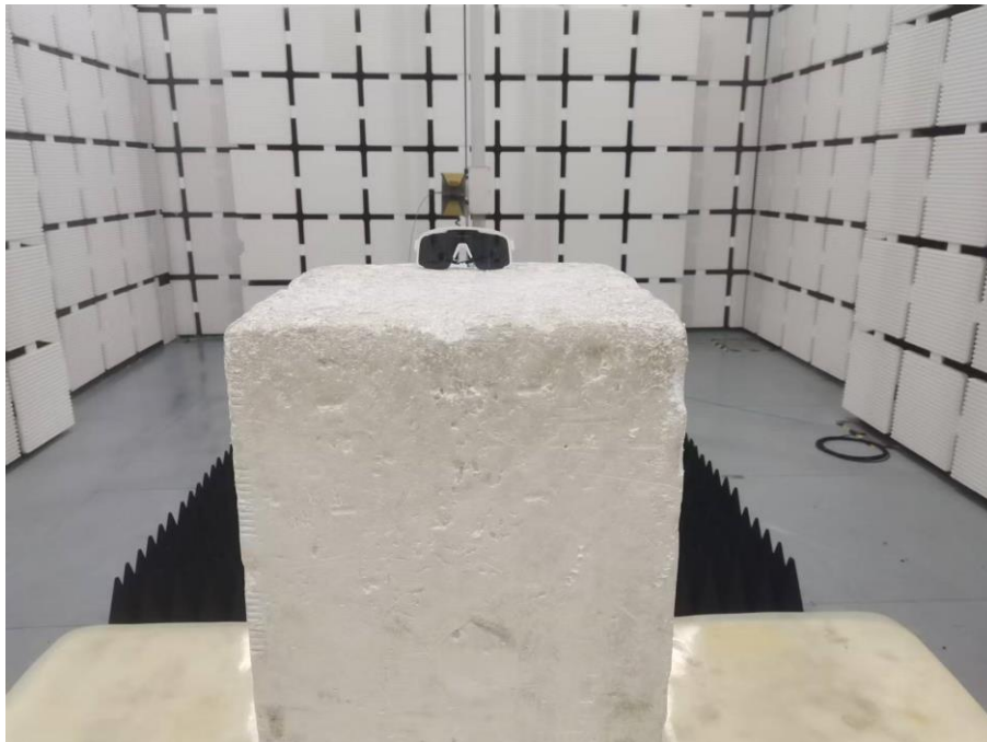
Set-up for Radiated Spurious Emission, Above 1GHz
