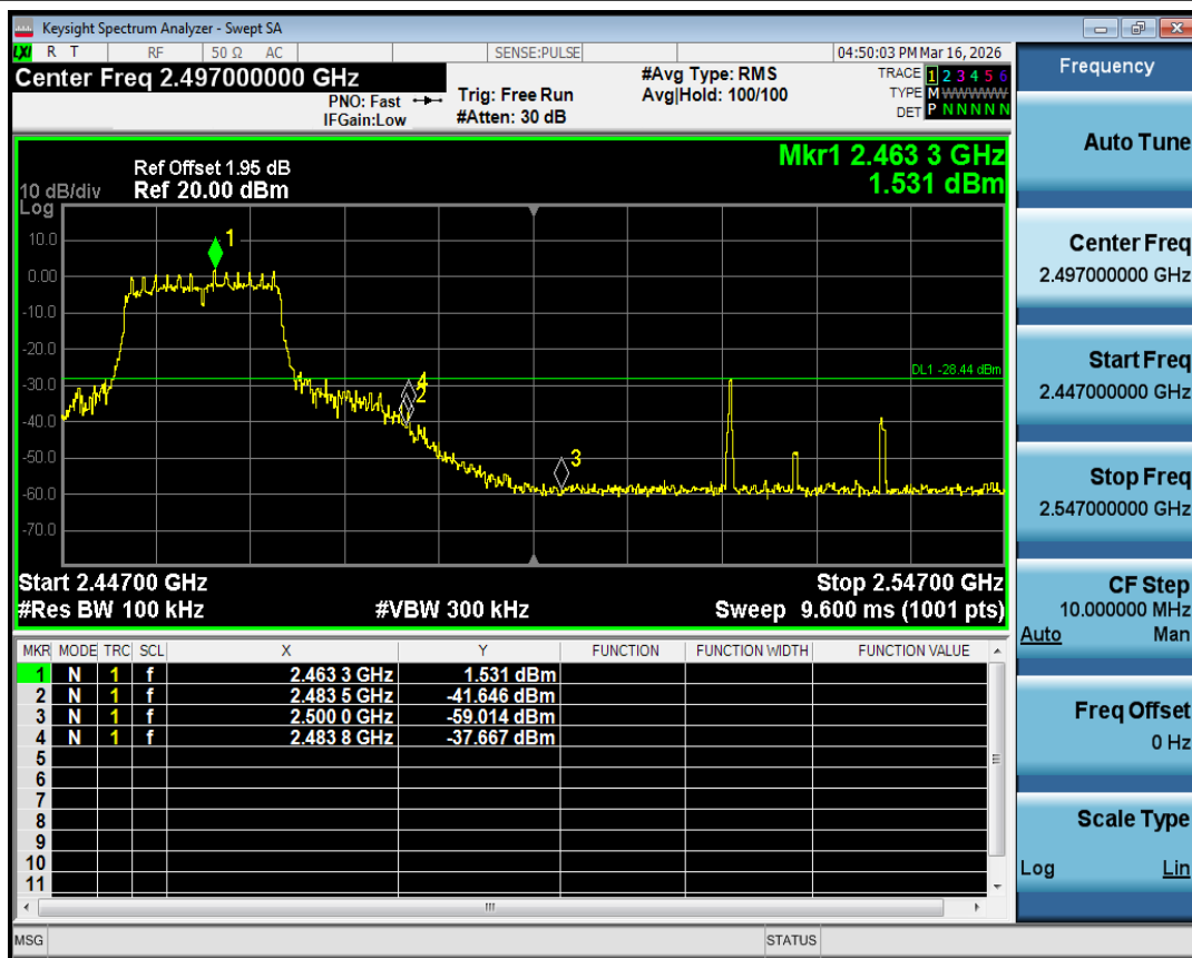
Band Edge NVNT g 2462MHz Ant1 Emission
