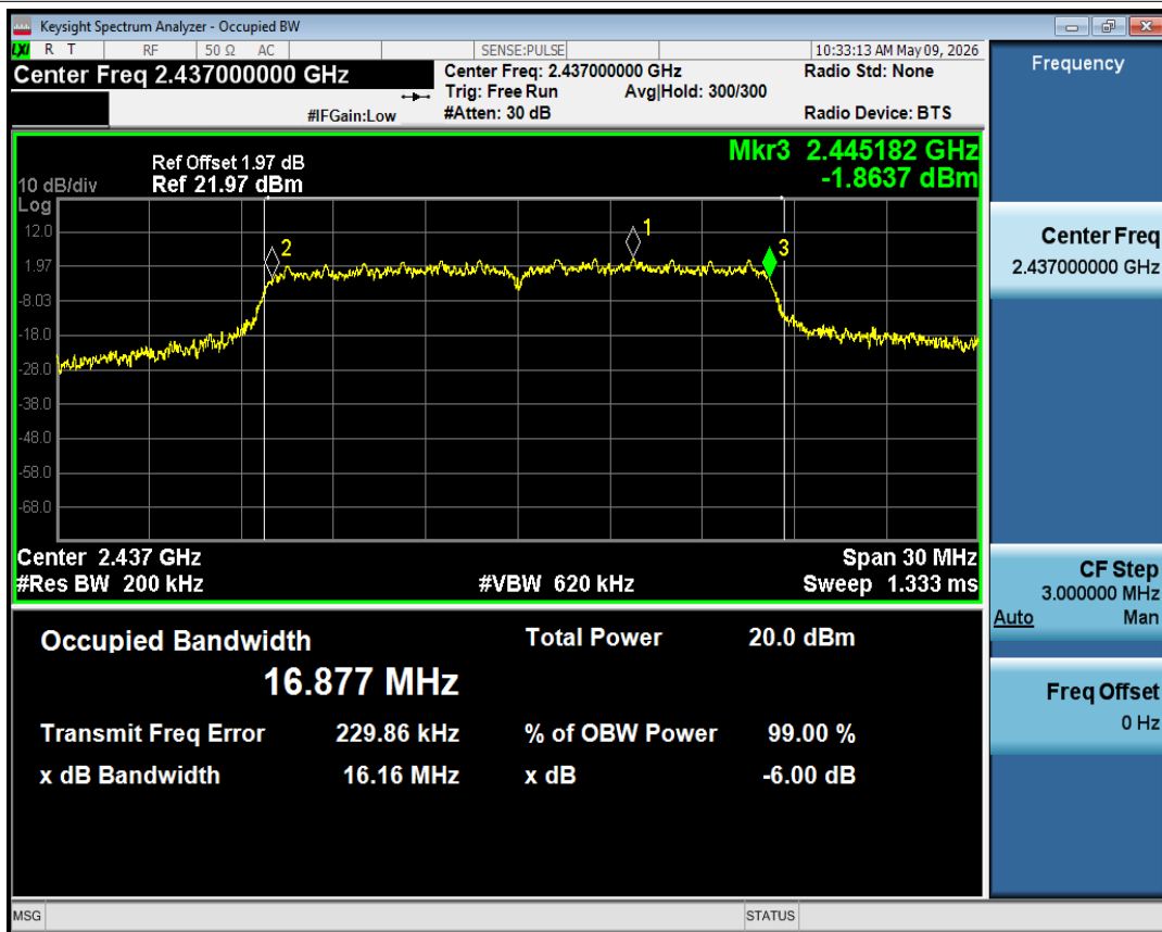
-6dB Bandwidth NVNT g 2437MHz Ant1
