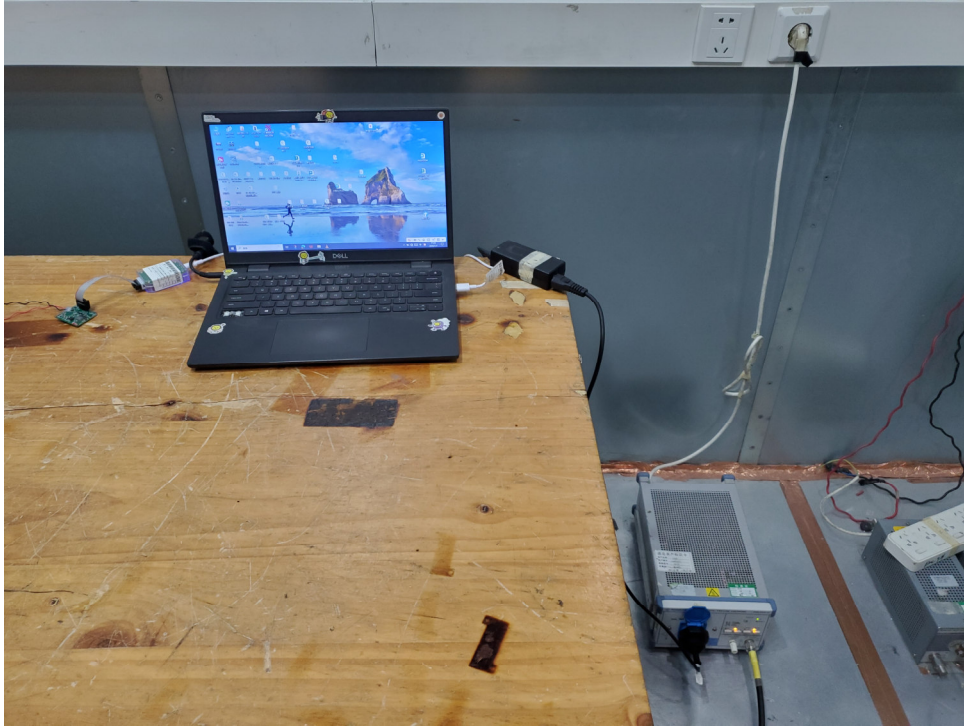
Picture 2 Conducted Emission Test Setup
